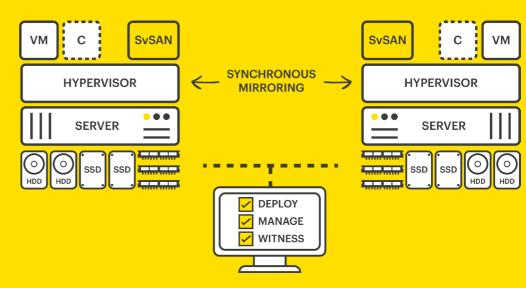
Fig. 1: A typical two-node SvSAN configuration
