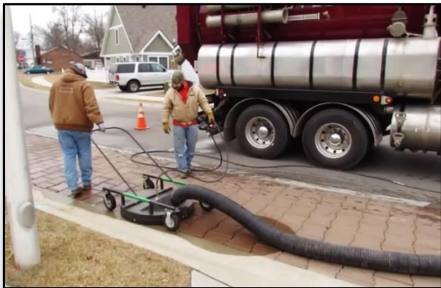
Combination Sewer Truck with 1,500 gallon water tank
