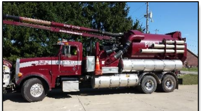
Combination Sewer Truck with 1,500 gallon water tank
