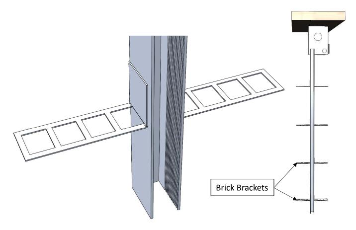
**Step 2:** Slide 3-4 Brick Brackets on to U-channel.
