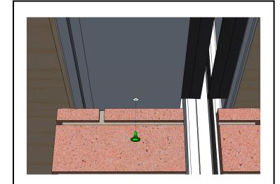
**Step 9:** Secure bottom at both ends of cover with tek screw.
