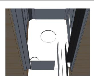
**Step 7:** Plumb and mount BuilderBrackets and U-channel on both ends. Bracket may need to be rotated and slid into place.
