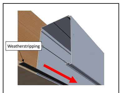
**Step 6:** Slide weatherstripping into back and bottom pieces. Some items omitted for clarity.
