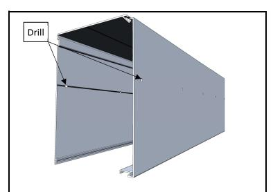
**Step 4:** Drill mounting holes in back and front of canister. Hinge front cover.
