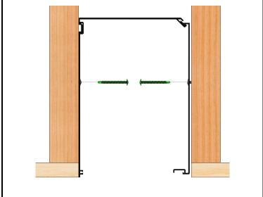
**Step 5:** Mount back, top and front of canister through drilled holes, flush with the ceiling.
