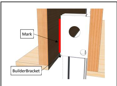
**Step 2:** Plumb U-channel and BuilderBrackets. Mark LVL on back side of BuilderBrackets on both ends of opening.
