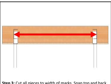
**Step 3:** Cut all pieces to width of marks. Snap top and back together. Some items omitted for clarity.
