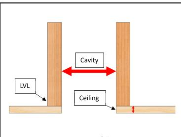
**Step 1:** Ensure cavity width is 7 3/4" and determine ceiling thickness.
