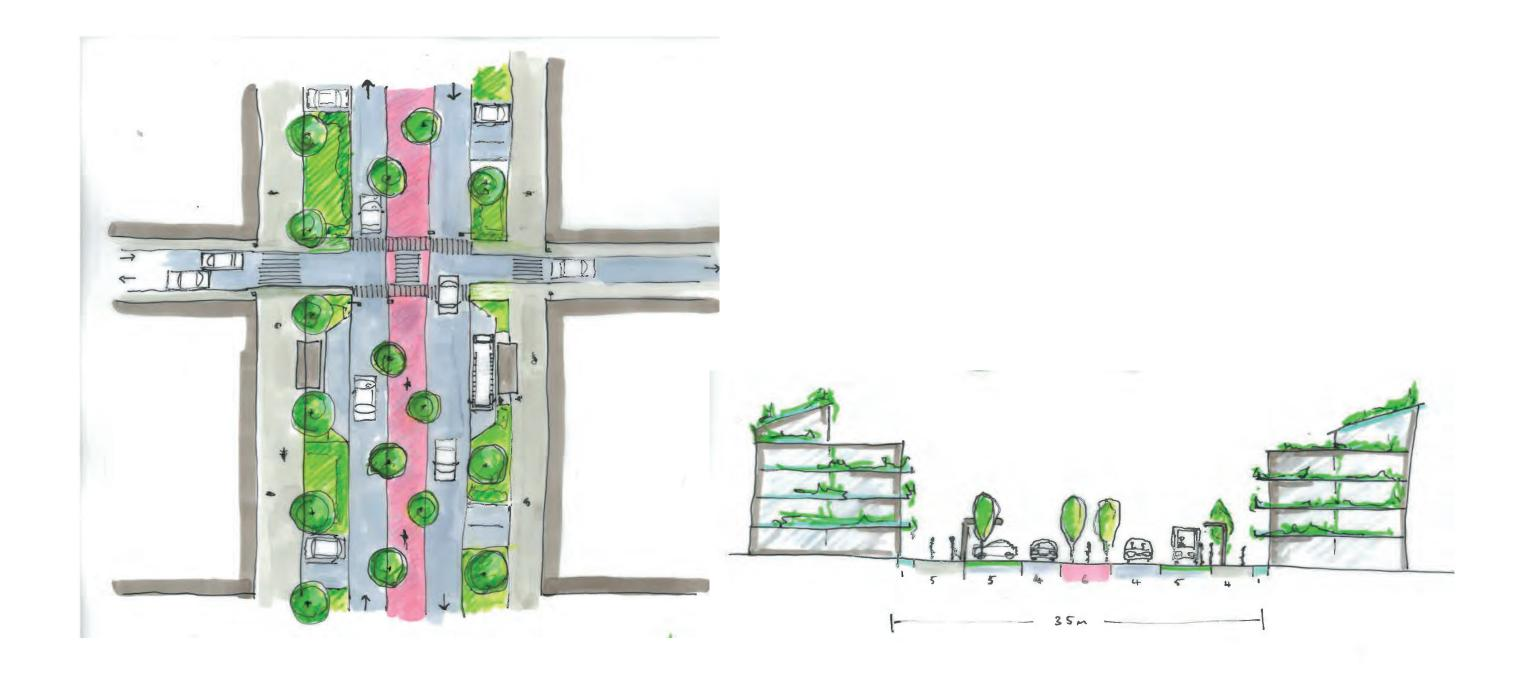
Figure 4.3 Illustrative High Street Cross Section: Short-term Arrangement
