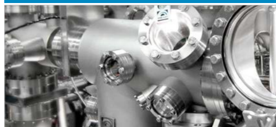
Reorientation chamber for STM
