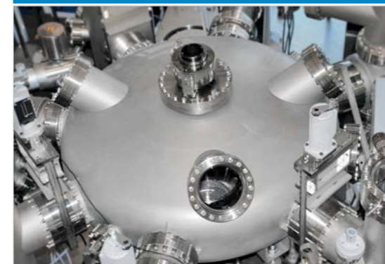
Semi automatic distribution chamber for 3" samples
