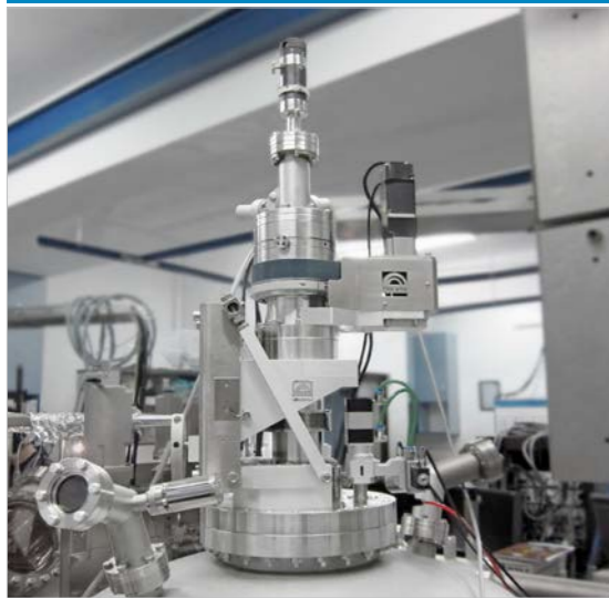
3" 1400°C 2 axes manipulator
