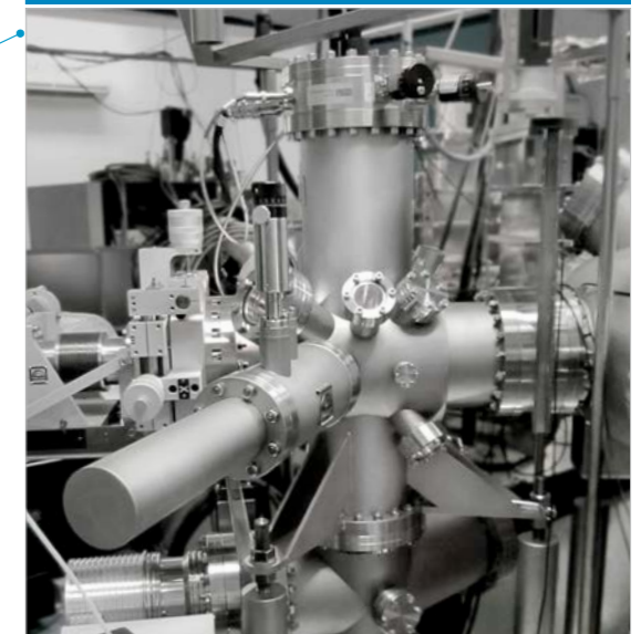
Preparation chamber with 1700°C heating stage
