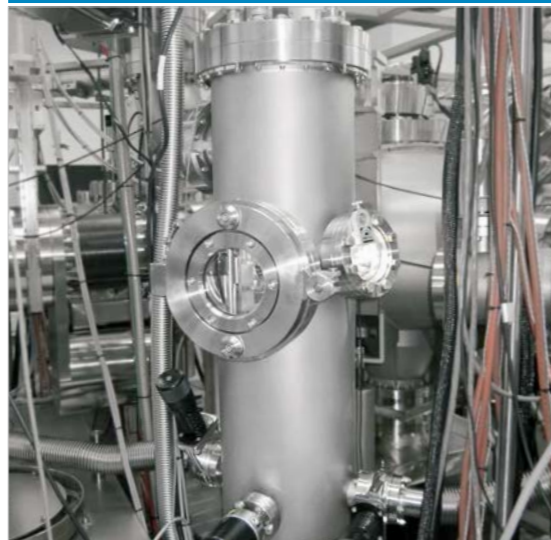
Load-lock chamber with storage
