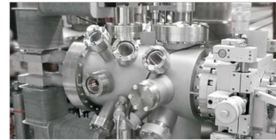
MOKE chamber for Kerr effect measurement
