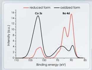
A catalyst sample - carbon sample coated with cobalt oxide  $Co_3O_4$  and barium carbonate  $BaCO_3$ , was examined just after impregnation. Co 3s and Ba 4d XPS spectra were obtained: black line marked as oxidized form of the catalyst. XPS analysis shows a considerable share of cobalt in the surface layer (in the form of oxide). There are only few barium compounds in this layer.
