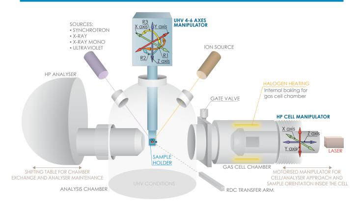
ANALYSIS MODULE GEOMETRY | SAMPLE IN HP CONDITIONS
