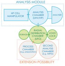
The heart of the system is the analysis module that is based on the high pressure analyser and a gas cell concept designed by PREVAC. HP cell manipulator design allows for sample heating by IR laser illumination (the sample temperature over 800 °C is reachable within the cell), resistive heating (up to 700 °C) and  $LN_2$  cooling.
