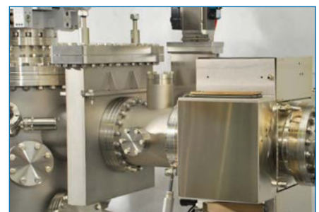
LN 2 cold trap between MBE chamber and pumping system.
