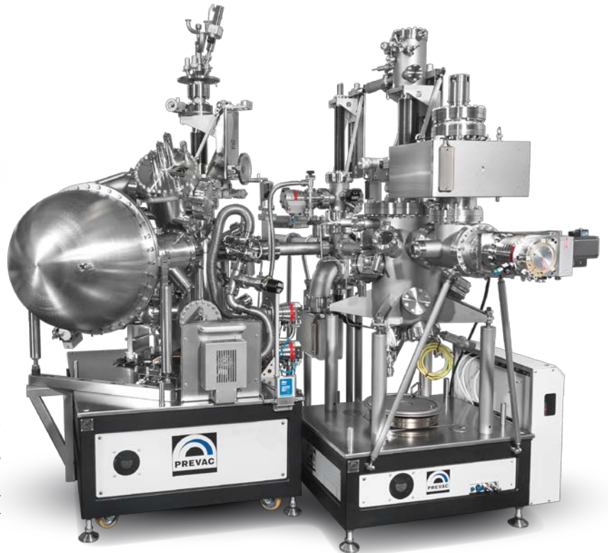
Multi-technique photo emission UHV system for super resolution ARPES measurements with integrated MBE chamber.
