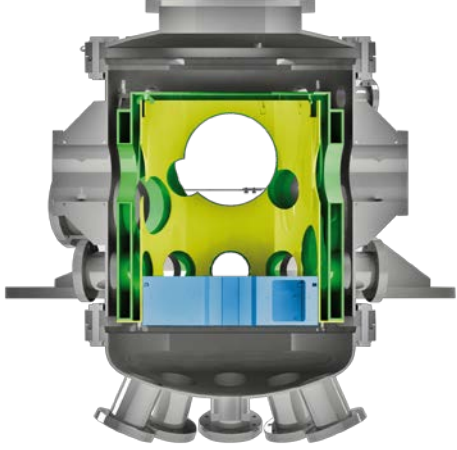
Arrangement of the cryo-panel, shroud and liner.
