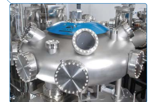
Radial distribution chamber
