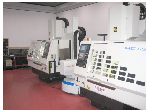
System 3R Automation LH Control Roku provides side by side installation Available on HC-658II only
