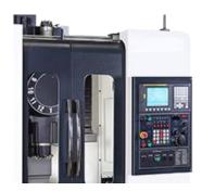
The DTC Line of Drill Tap Machining Centers features the FANUC OiMF CNC Control. AICCII with 400 block look ahead is built into the base control package. This standardly equipped control package helps to unlock the full potential of the high speed machine design.
