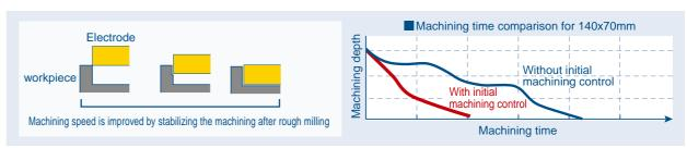
Machining time is reduced up to 40% by optimizing smoothing of simultaneous 2 or 3 axes operation and speed/acceleration control
