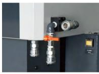
Sprays dielectric fluid between the workpiece and electrode during pitch machining
