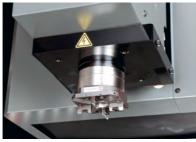
Clamp spindle side holder with air chuck (photo shows EROWA-ITS chuck specications)
