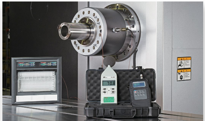
Spindle vibration and noise checking.
