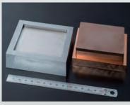
Automatic depth recognition and stable servo control using "Maisart" make uniform surface finish.
