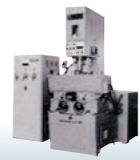
1964 DM201 Production started 1964 Thyristor power supply Hydraulic servo system
