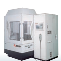
2001 MA2000 Began shipment in May 2001 Equipped with thermal displacement compensation
