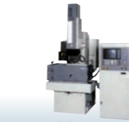
1986 M25KC4 Began shipment May 1986 Equipped with ultralow-wear power supply (slope control system)
