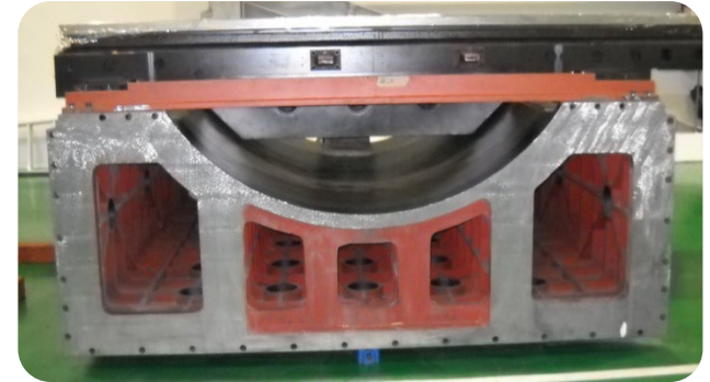
Underside of Column
