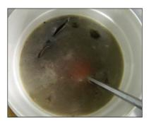
**4.** This is the water after a 30-40 minute soak with periodic agitation. You can see the dissolved fats and oils on the surface.
