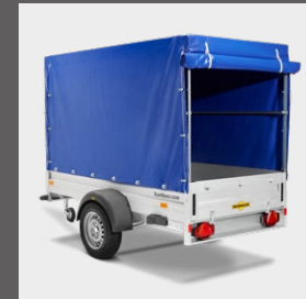
Tarpaulin and frame, load height 1000/1300/1600/1800 mm (version depends on model)
