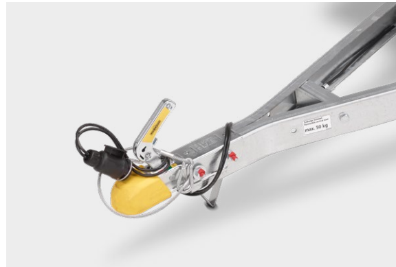
Hot-dip galvanized V drawbar with transverse strut
