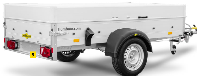
Optional aluminium loading ramps can be pushed into the underrun protection
