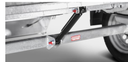
Tipping body (on the tipping HA) with shock absorber support
