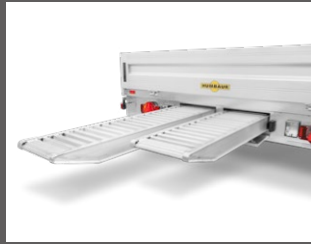
Aluminium-Ramps (up to 1.9t load capacity / length 2465 mm; up to 2.3t load capacity / length 2230 mm; up to 2.8t load capacity / length 2650 mm)
