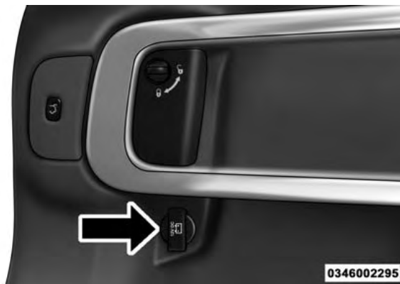
Rear Power Outlet
