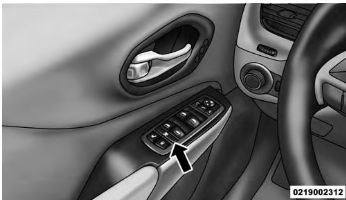
Window Lockout Switch
