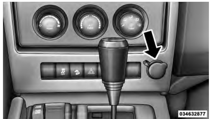
Front Power Outlet
