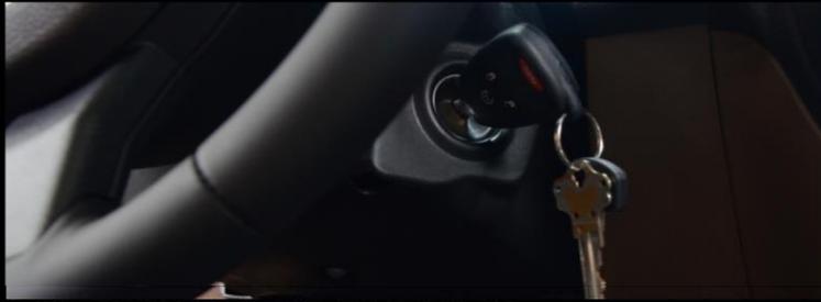
2013 JK is devoid of marking for On/O . Photo above shows ignition in OFF position.
