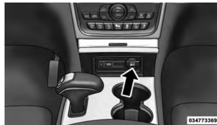
Front Power Outlet
