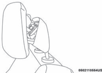
Active Head Restraint (AHR) Deployed
