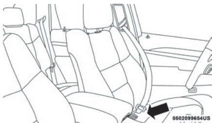
Inserting Latch Plate Into Buckle
