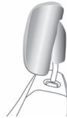
Active Head Restraint (Normal Position)
