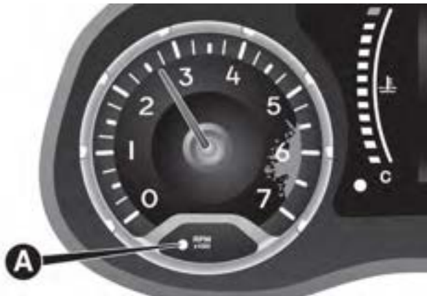
Vehicle Security Light Location
