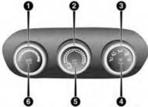
Manual Temperature Controls (MTC)
