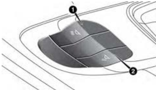
Courtesy Light Switches
