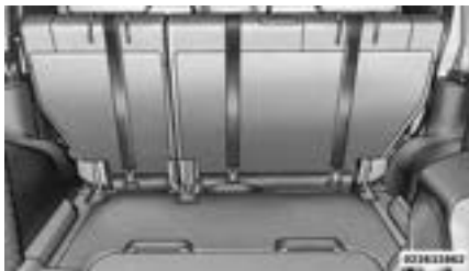
Tether Strap Mounting (Four-Door Models)
