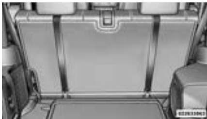
Tether Strap Mounting (Two-Door Models)
