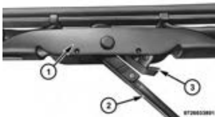
Wiper Blade With Release Tab In Locked Position
