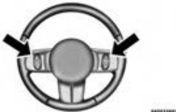
Remote Sound System Controls (Back View Of Steering Wheel)
