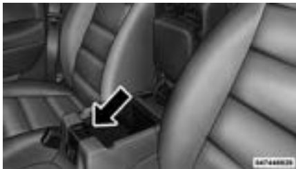
Center Console USB/AUX Connector Port
