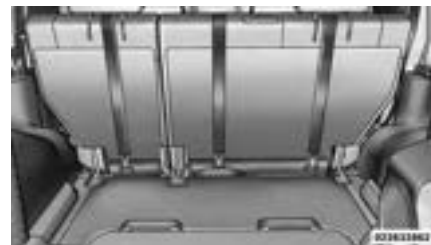
Tether Strap Mounting (Four-Door Models)
