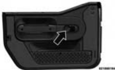
Manual Door Lock (Half Doors)
