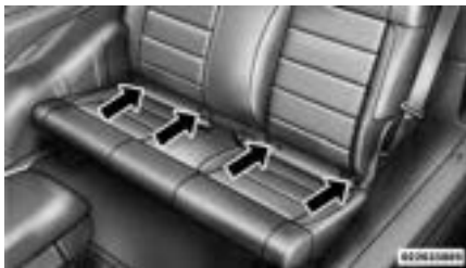
Latch Anchorages (Two-Door Models)
