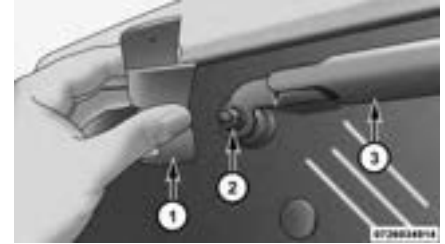
Wiper Arm With Pivot Cap Removed
