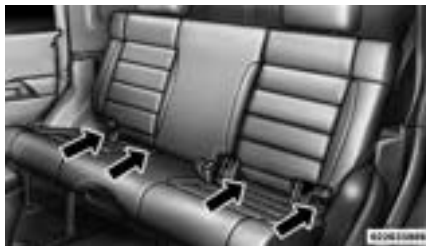
Latch Anchorages (Four-Door Models)
