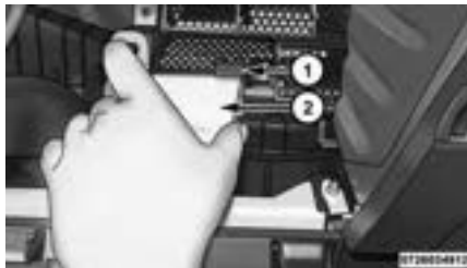
Air Filter Access Door Open
