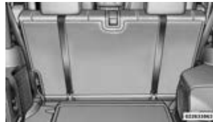
Tether Strap Mounting (Two-Door Models)
