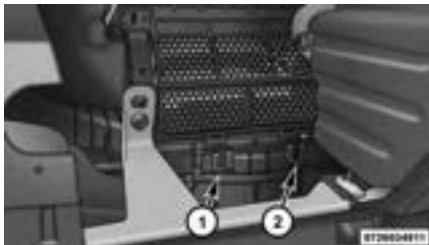
Air Filter Retaining Tabs
