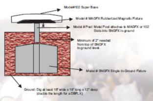
MAGBASE bases, when installed with the magnetic anchors, are designed to disengage on impact from an improper or fast slide, thus preventing severe injury in most cases.
