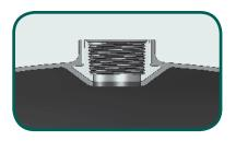
Top connection with stainless steel reinforcement ring is encapsulated in a precision omolded dome to withstand the harshest environments.
