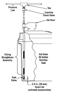
The pump may be mounted on a molded tank, 15-gallon tanks (part no. 34054) and 35-gallon tanks (part no. 34055) are suitable for pump mounting.
