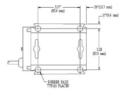
Figure 2: Rubber Pad Replacement
