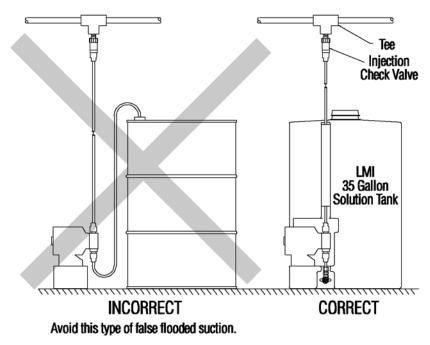
Figure 3: Flooded Suction Installation
