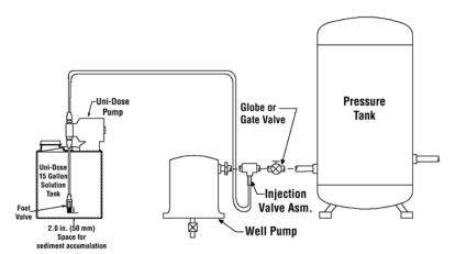
Figure 7: Well Pump System
