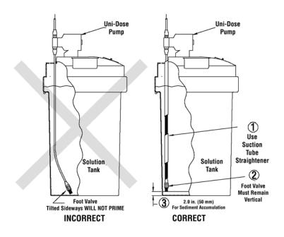
Figure 9: Foot Valve Position
