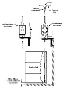
Figure 4: Wall Bracket Mount
