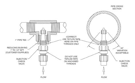
Figure 10: Typical Injection Check Valve Installation
