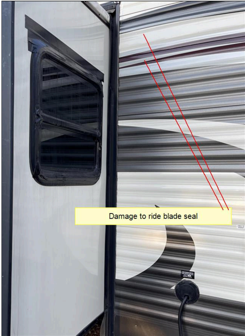
right side of slideout sesal blade damaged
