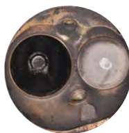
Cylinder head after one P.i. treatment.
