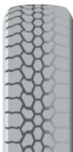
Wear on one side only □ Poorly aligned wheel
