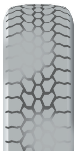
Uneven wear □ Poorly balanced wheel
