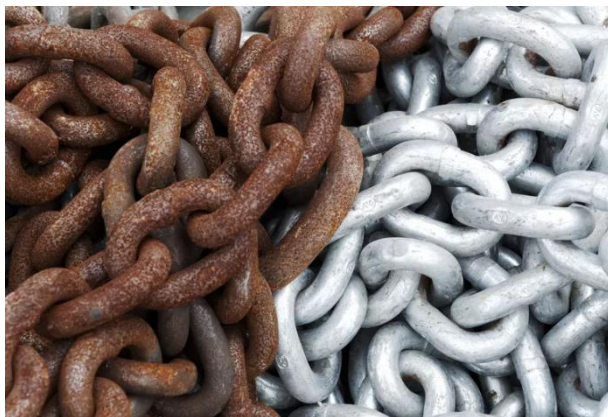
Figure 3. Example of a chemical change as metal chains rust over time. The chains on the left have rusted. The chains on the right have not because they have a special coating that prevents them from rusting. Source: photostock-israel/getty images
