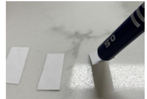
Plastic pen lifting up paper after rubbing the plastic against hair.
