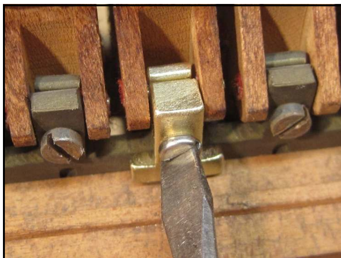
Repair clip for broken tongue being installed.
