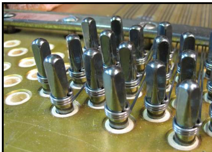
New tuning pins and strings being installed.
