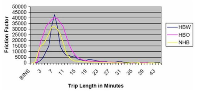
FIGURE 2 Friction factors for HBW, HBO, and NHB trips. (Source: Cambridge Systematics, Inc., 2004.)
