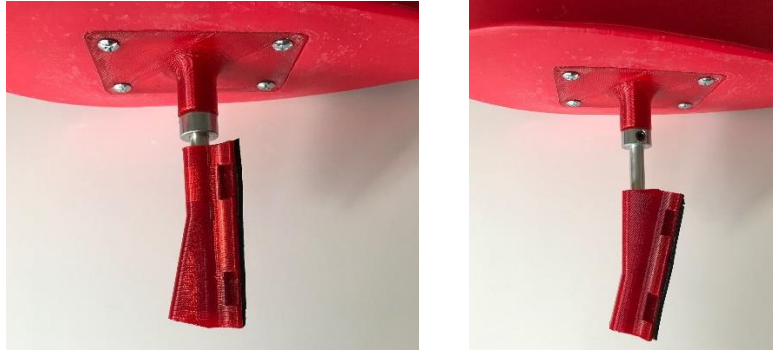
Above: The rotating shaft screws into either end of the Lower Bracket depending on orientation of the mast or spar on which it is mounted. Left: lower bracket position for vertical masts (Zuma, etc.). Right: lower bracket position for inclined masts / spars (Sunfish, Snark, Laser and similar)
