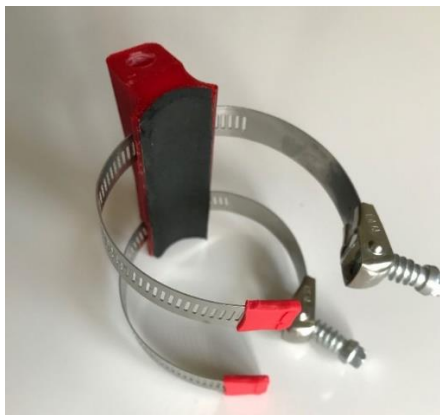
Above left: upper bracket sub-assembly screwed into recess on underside of the float. Middle: trimmed stainless-steel bands inserted in the slots in the lower bracket. End caps prevent cuts from the sharp ends of the thin metal bands. The caps must be removed temporarily for installation or removal of the bracket from the mast / spar. Right: Lower bracket attached to Snark-sized (0.75" diameter) tube with reusable zip ties (8.3" GripLockTies shown).
