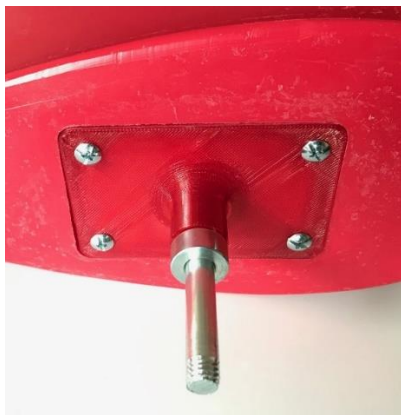
Above left: upper bracket sub-assembly screwed into recess on underside of the float. Middle: trimmed stainless-steel bands inserted in the slots in the lower bracket. End caps prevent cuts from the sharp ends of the thin metal bands. The caps must be removed temporarily for installation or removal of the bracket from the mast / spar. Right: Lower bracket attached to Snark-sized (0.75" diameter) tube with reusable zip ties (8.3" GripLockTies shown).
