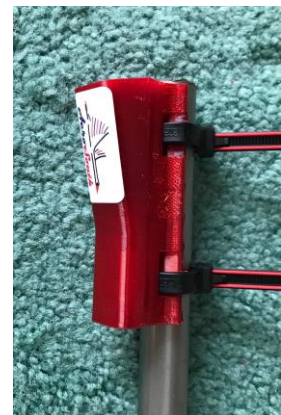
Above left: upper bracket sub-assembly screwed into recess on underside of the float. Middle: trimmed stainless-steel bands inserted in the slots in the lower bracket. End caps prevent cuts from the sharp ends of the thin metal bands. The caps must be removed temporarily for installation or removal of the bracket from the mast / spar. Right: Lower bracket attached to Snark-sized (0.75" diameter) tube with reusable zip ties (8.3" GripLockTies shown).
