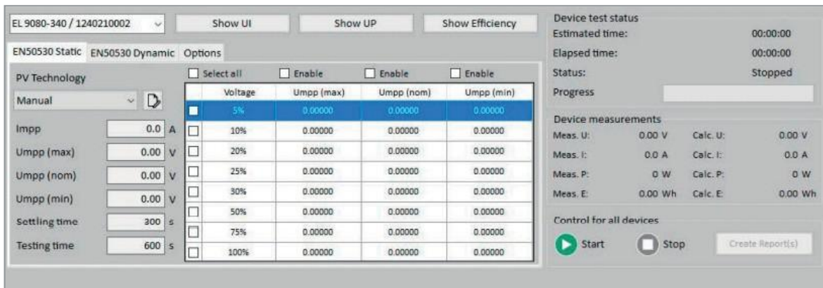
Figure 9 Power Control software window for the solar array static test
