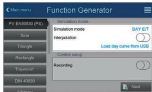
Figure 7b Window showing options for the simulation mode, interpolation of transitions, and data storage
