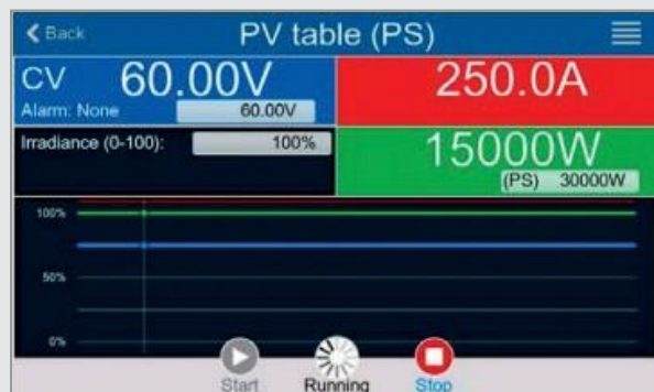
Figure 5 Solar panel main display window showing the measured output parameters, the controlled variable, solar irradiance in this display, and how close the panel is operating to its maximum power point.
