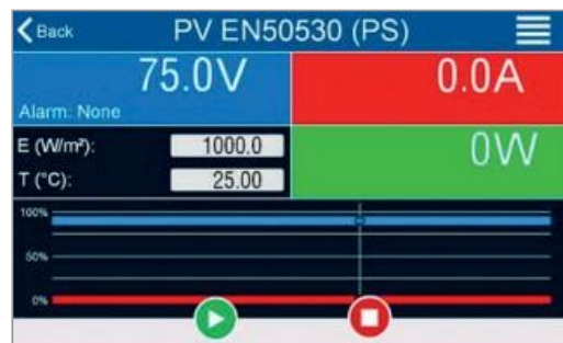
Figure 8 PV EN50530 operating display window showing measured parameters, the controlled variables, and the output relative to the maximum power point.
