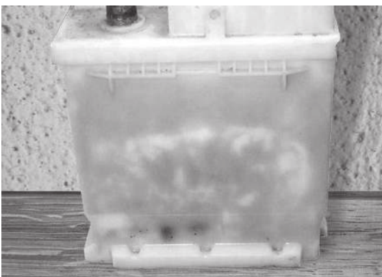
Figure 1 – Picture of battery with deep discharge and sulphation
