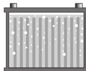
Figure 2 – Without acid stratification
