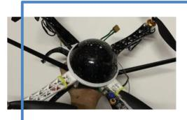
Drone Developed by Techno Hub to transport medicines payload 2 kg
