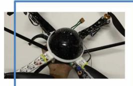
Drone Developed by Techno Hub to transport m dicines payload 2 kg
