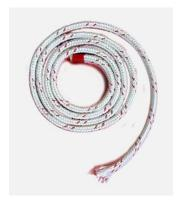
FIPRON CORD is a cord type of fire extinguisher. It is a new generation of a fire suppression products consisting of composite materials having a mixture of microcapsules with a heating compound. Under the effects of a fire and a temperature of 170 °C at any of its points, an initiation of the heating compound occurs with subsequent chemical reaction throughout its length. The reaction results in the bursting of all microcapsules of the extinguishing agent.
