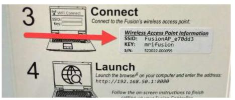
One of the unique things about a Fusion robot is that, as well as acting as a robot, it also acts as a server with an inbuilt Wi-Fi link. Laptops, desktop PCs, tablets or smart phones can connect to the Fusion robot using this Wi-Fi link. It is almost as if the Fusion robot is its own Wi-Fi hotspot, except that the Wi-Fi connection is not to the
