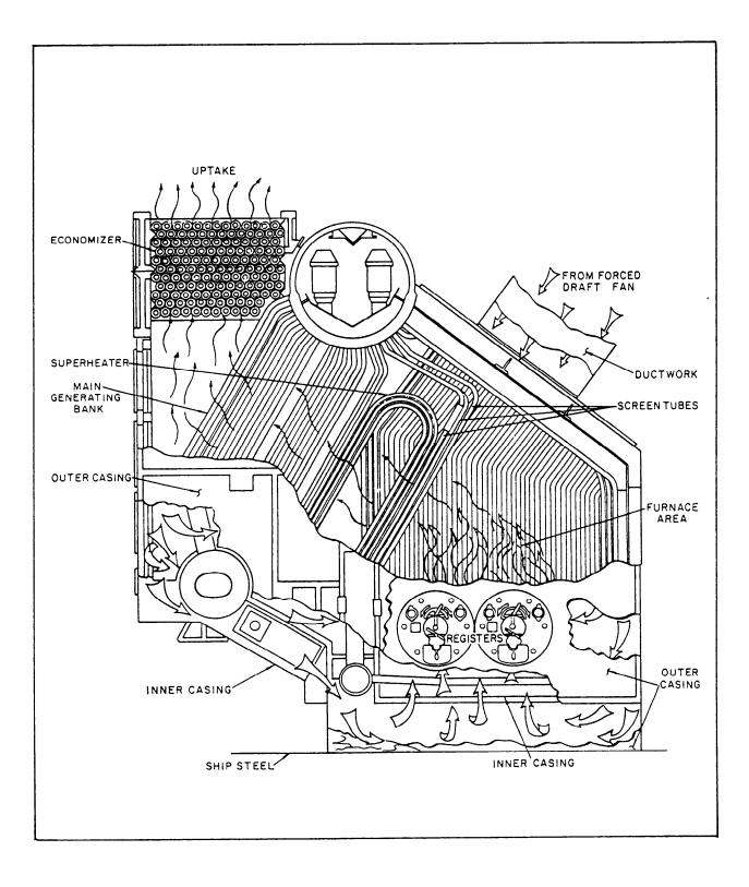
Figure 15-12.—Combustion air and gas flow.
