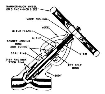
Figure 10-9.—1500-pound pressure seal bonnet globe valve.
