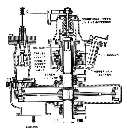
Figure 2-27.—Main condenser circulating pump turbine.
