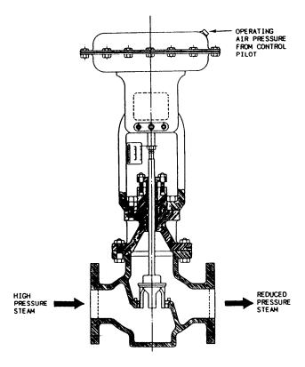
Figure 10-22.—Diaphragm control valve (downward seating).
