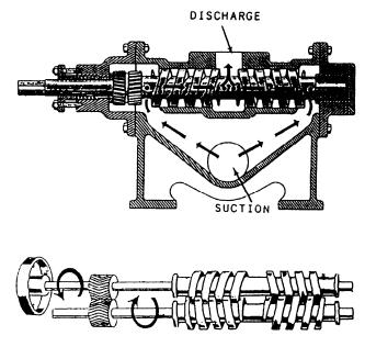
Figure 5-20.—Positive displacement, double-screw, low-pitch pump.
