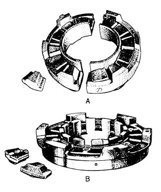
Figure 3-13.—Pivoted-shoe thrust bearing.
