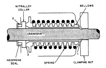
Figure 11-8.—Rotating bellows seal.
