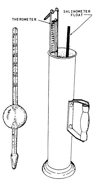
Figure 9-13.—Salinometer and sampling pot.
