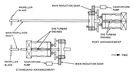
Figure 3-23.—Main propulsion system
