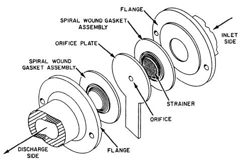
Figure 10-30.—Orifice-type steam trap assembly.
