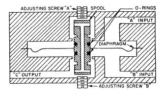
Figure 17-13.—High signal selector.
