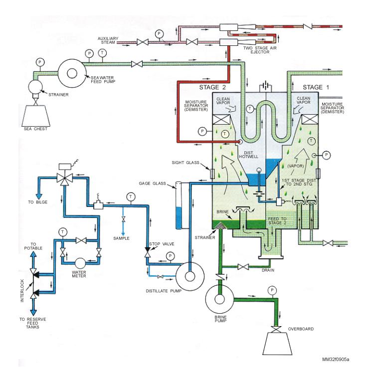
Figure 9-5.—Two-stage, flash-type distilling plant 12,000 gpd capacity.
