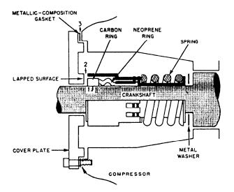
Figure 11-6.—Rotary seal.
