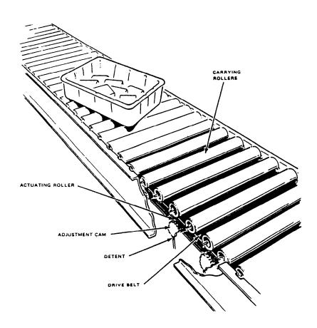
Figure 14-9.—Powered roller conveyor.
