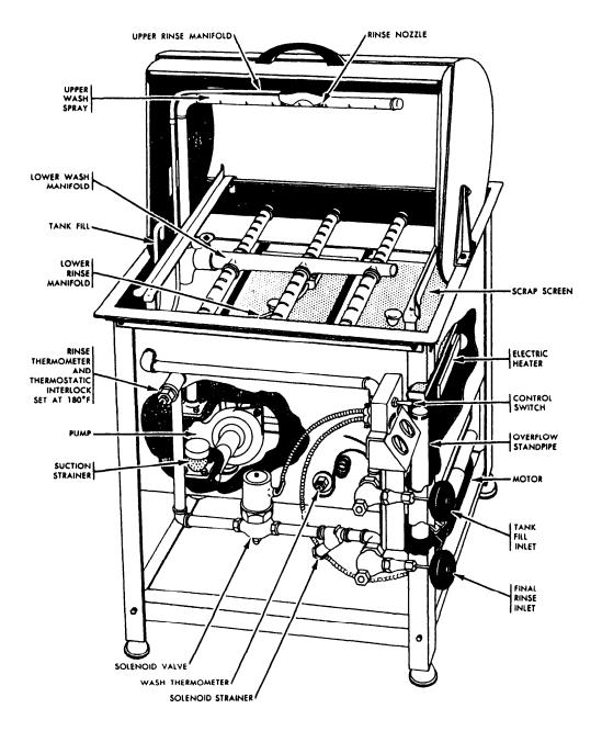
Figure 14-13.—Typical semiautomatic single-tank dishwashing machine.
