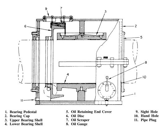
Figure 3-16.—Line shaft bearing (disc oiled).
