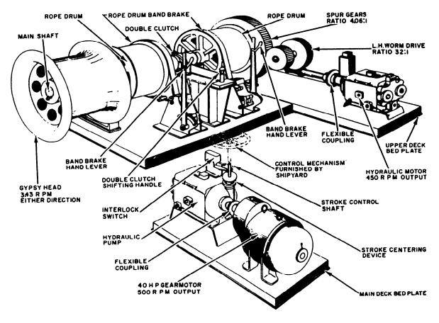
Figure 14-3.—Electrohydraulic winch unit.
