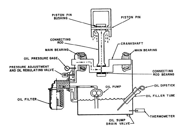
Figure 13-8.—Lubricating oil system of a low-pressure air compressor.
