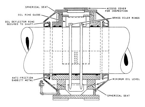
Figure 3-15.—Main line shaft bearing (ring oiled).
