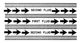
Figure 6-1.—Parallel flow in a heat exchanger.
