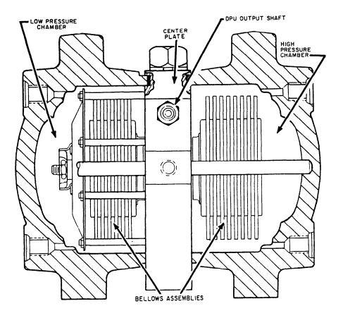
Figure 16-20.—Differential Pressure-Sensing Unit (DPU).
