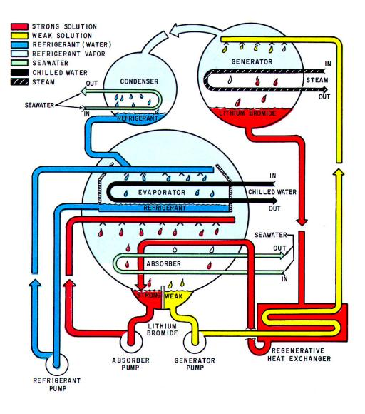
Figure 12-8.—Basic absorption cycle.
