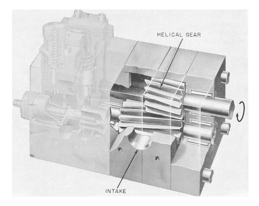
Figure 5-18.—Helical gear pump.
