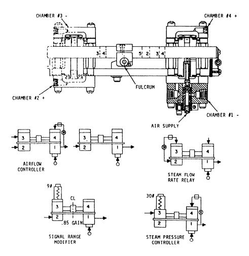
NOTE: A SPRING BARREL AND SPRING ASSEMBLY CAN BE ATTACHED TO CHAMBERS 2, 3, OR 4 TO INDUCE A MECHANICAL INPUT FORCE.
