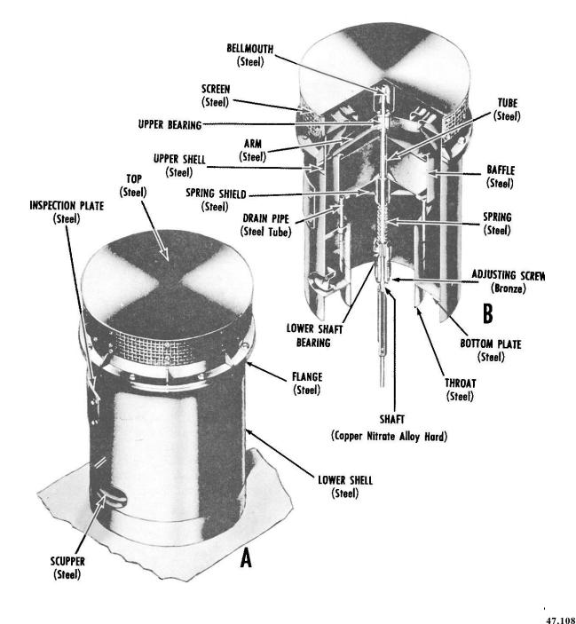
Figure 12-4.—Waterproff ventilators: A. Exterior view. B. Cutaway view.
