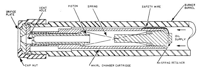
Figure 16-25.—Vented-plunger atomizer.
