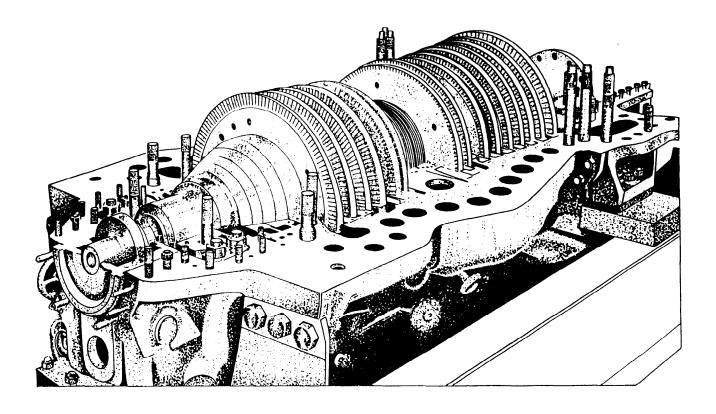
Figure 2-22.—Turbine cylinder base with rotor installed, viewed from thrust end.
