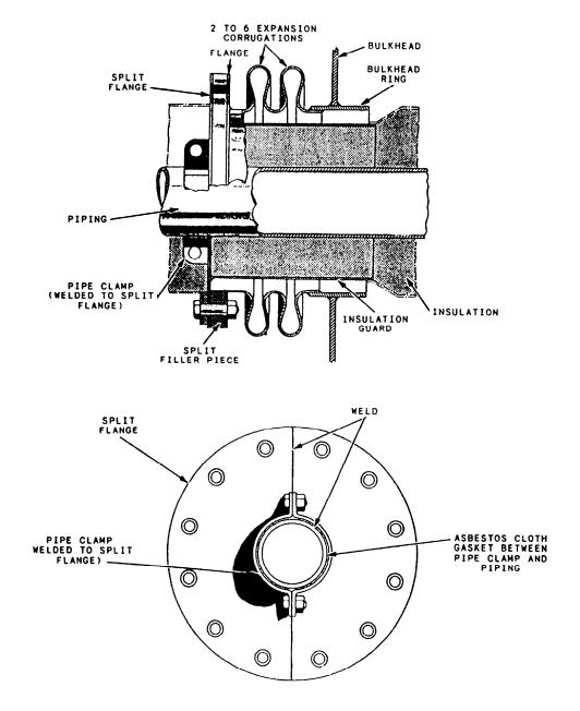
Figure 10-6.—Corrugated bulkhead expansion joints, showing details of installation.
