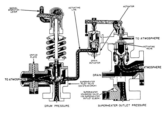
Figure 16-24.—Three-valve superheater outlet safety valve assembly.
