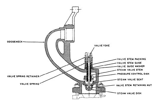
Figure 16-13.—Cross-sectional view of a rotary soot blower.
