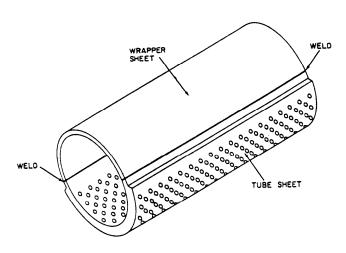
Figure 15-1.—Boiler steam drum.
