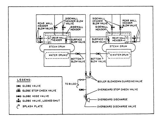
Figure 16-16.—Boiler blow piping.
