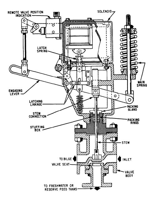
Figure 9-6.—Three-way solenoid trip valve.
