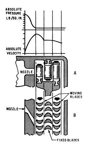
47.182 Figure 2-7.—Pressure-velocity relationships in a velocitycompounded impulse turbine.
