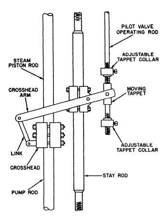
Figure 5-13.—Valve operating assembly.
