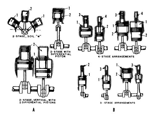
47.153 Figure 13-3.—Air compressor cylinder arrangements: (A) Low- and medium-pressure compressors; (B) High-pressure compressor.
