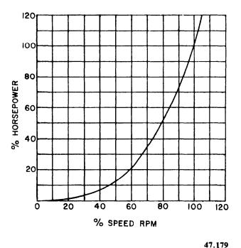
Figure 2-2.—Horsepower-speed cube relationship.
