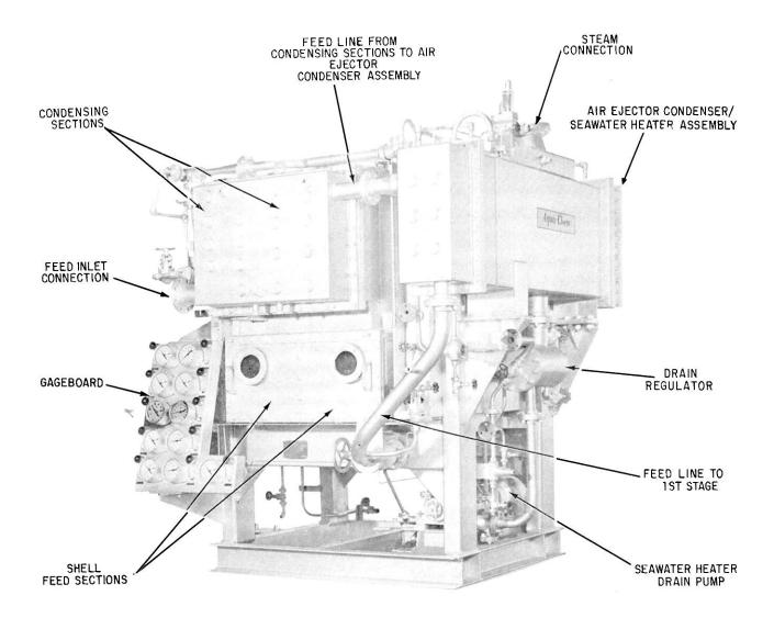
Figure 9-4.—Two-stage, 12,000 gpd flash-type distilling plant.
