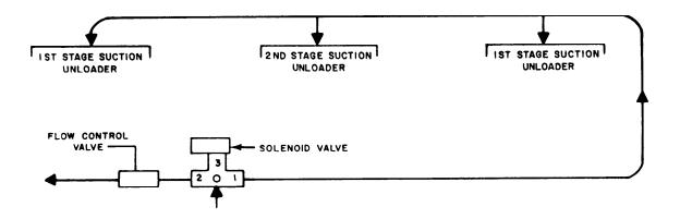
Figure 13-20.—Unloaded system from the oil-free low-pressure air compressor.
