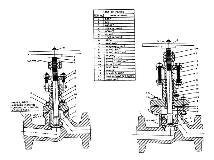
Figure 16-10.—Stop-check valves.
