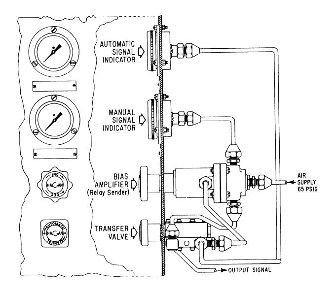
Figure 17-14.—Boiler four-way A/M station.
