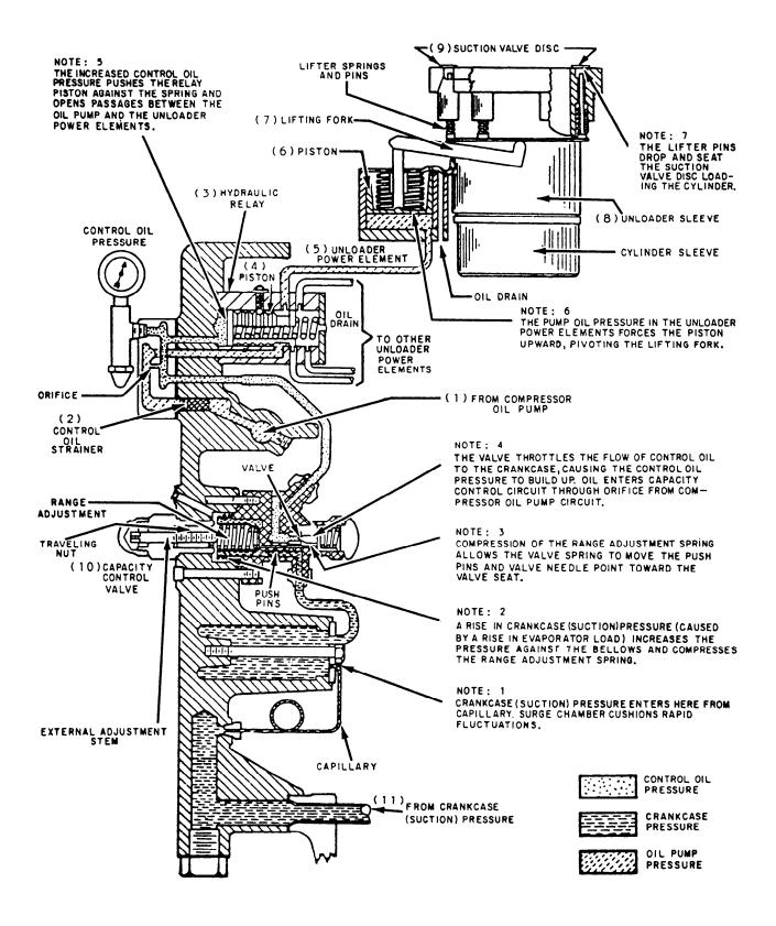
Figure 11-10.—Capacity control system.
