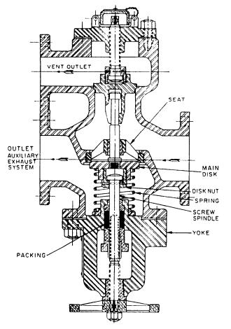
Figure 5-23.—Combined exhaust and relief valve.
