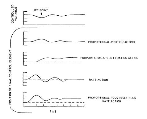
Figure 17-9.—Proportional plus reset plus rate action.
