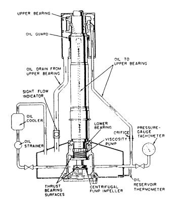
Figure 5-28.—Lubrication system for a vertical forced draft blower (oil supplied through hollow shaft and through external supply line).
