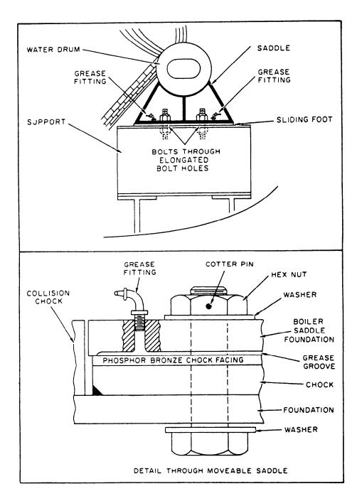
Figure 15-11.—Boiler saddle, support, and sliding feet.
