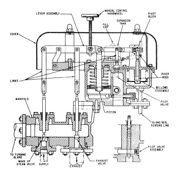
Figure 2-20.—Hydraulic type turbine gland seal regulator.
