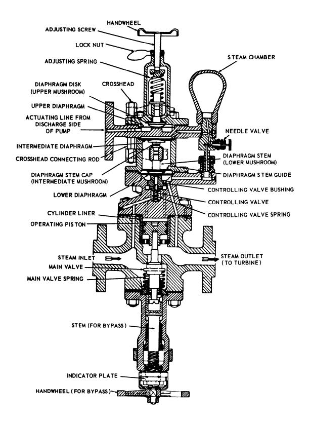
Figure 5-9.—Constant-pressure governor for main feed pump.
