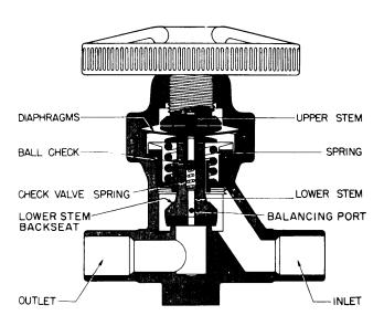
Figure 11-19.—Packless valve for refrigeration system.
