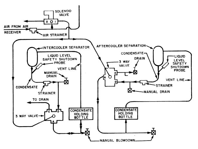
Figure 13-21B.—Condensate drain system.
