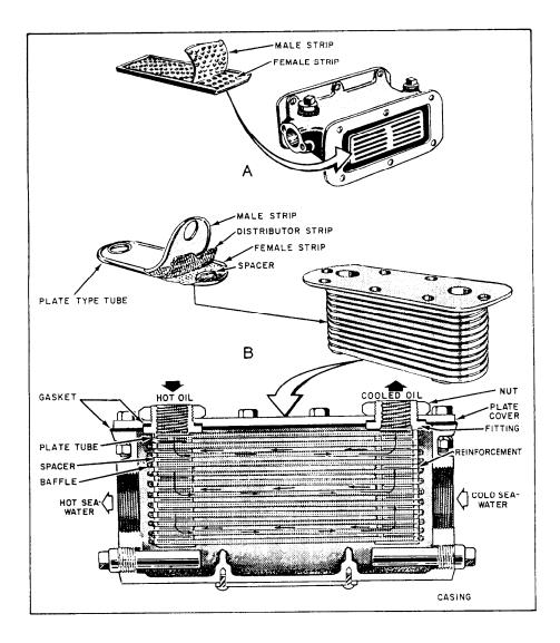
Figure 6-11.—Oil coolers for pumps. A. Strut-tube type. B. Plate-tube type.
