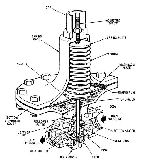
Figure 10-17.—Pressure-reducing (spring-loaded) valve.
