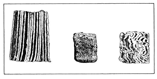
Figure 10-34.—Sectional views of corrugated ribbon packing after restructuring.
