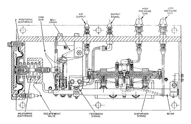
Figure 17-15.—Wind box airflow transmitter.
