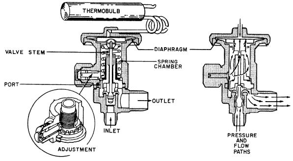
Figure 11-20.—Thermostatic expansion valve.
