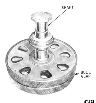
**Figure 3-5.—Bull gear assembly with shaft.**
