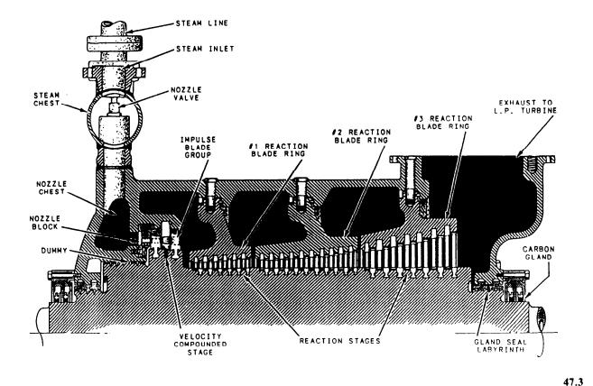
Figure 2-12.—Combination impulse and reaction turbine.
