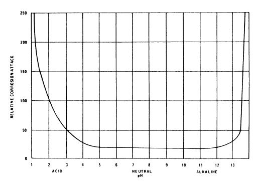
Figure 18-5.—pH effect on boiler metal corrosion.
