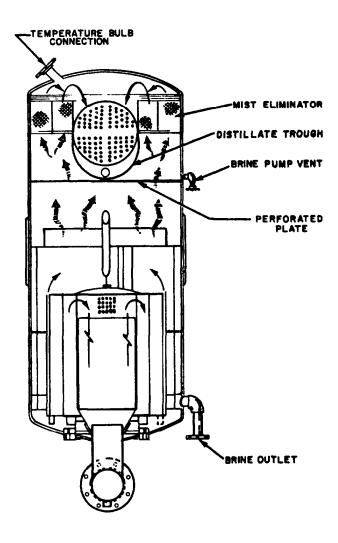
Figure 9-9.—Side view (cutaway) of vertical basket distilling plant.
