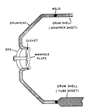
Figure 15-2.—Drumhead secured to steam drum.
