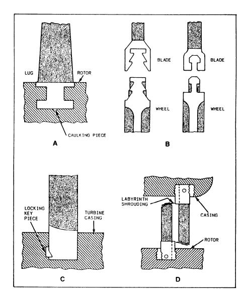
**47.16** Figure 2-21.—Methods of securing turbine blades: A. Straight circumferential dovetail. B. Inverted circumferential dovetail. C. Side-locking key piece. D. Sawtooth servation.
