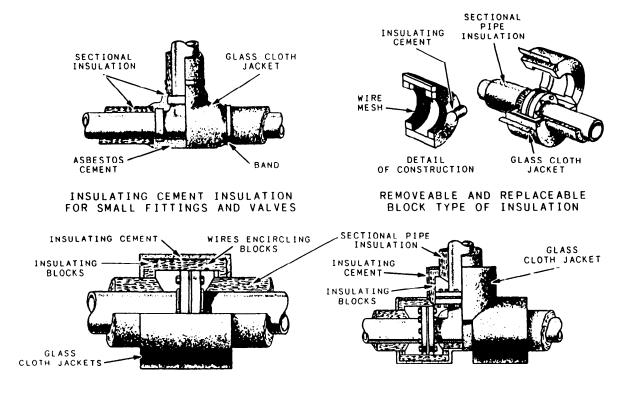
Figure 10-37.—Permanent-type insulation of pipe fittings, flanges, and valves.
