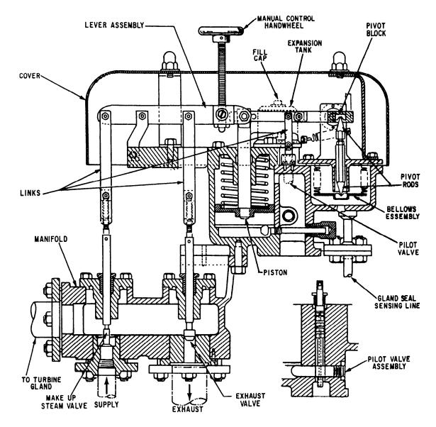
Figure 10-25.—Hydraulic steam seal regulator.
