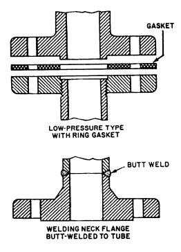
Figure 10-2.—Bolted flange piping joints.
