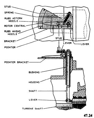
Figure 2-34.—Axial clearance indicator.
