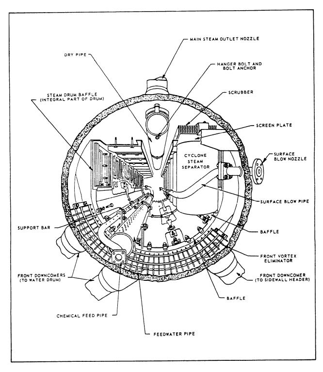
Figure 16-1.—Arrangement of internal fittings in a single-furnace boiler.
