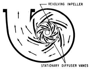
Figure 5-3.—Diffuser (volute turbine) pump.
