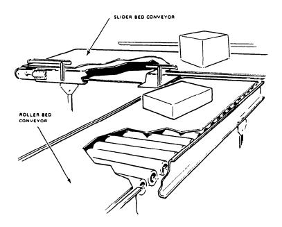
Figure 14-8.—Powered belt conveyor.
