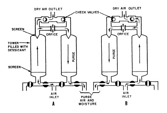
Figure 13-15.—Heat-les dehydrator.
