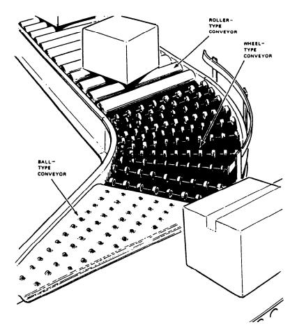
Figure 14-5.—Gravity conveyor.
