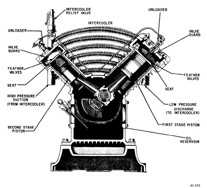
Figure 13-1.—A simple two-stage reciprocating low-pressure air compressor.
