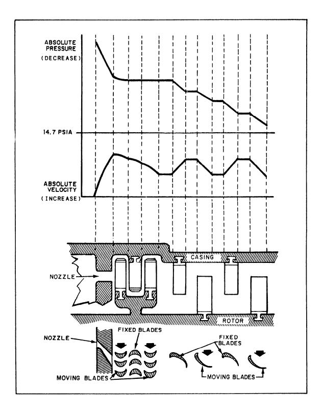
Figure 2-11.—Diagrammatic arrangement of combination impulse and reaction turbine showing pressure velocity relationships.
