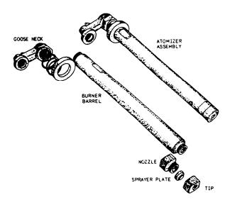
Figure 16-26.—Parts of a straight-through-flow atomizer assembly.
