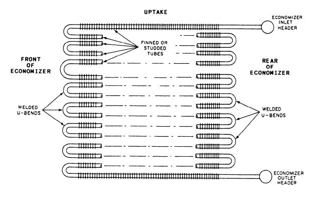
Figure 15-8.—Side view of economizer showing one element.
