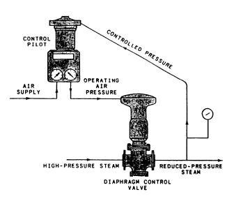
Figure 10-24.—Arrangement of control pilot and diaphragm control valve for supplying reduced steam pressure.
