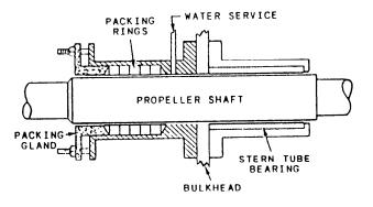
Figure 3-18.—Stern tube stuffing box and gland.
