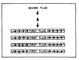
Figure 6-3.—Crossflow in a heat exchanger.
