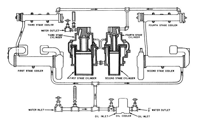
Figure 13-9.—Cooling water system in a typical multistage air compressor.
