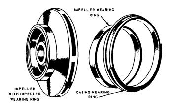
Figure 5-8.—Impeller, impeller wearing ring, and casing wearing ring for a centrifugal pump.
