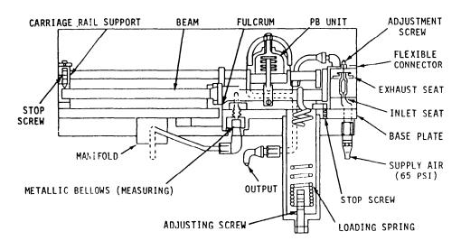
Figure 17-12.—Steam pressure transmitter.
