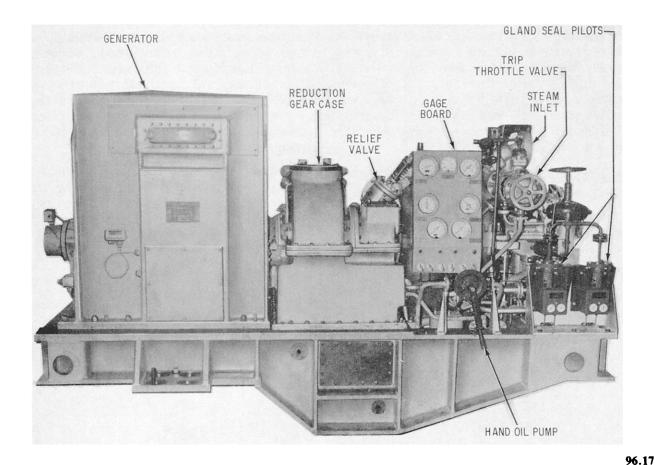
Figure 2-28.—750 KW a.c. turbine generator set.
