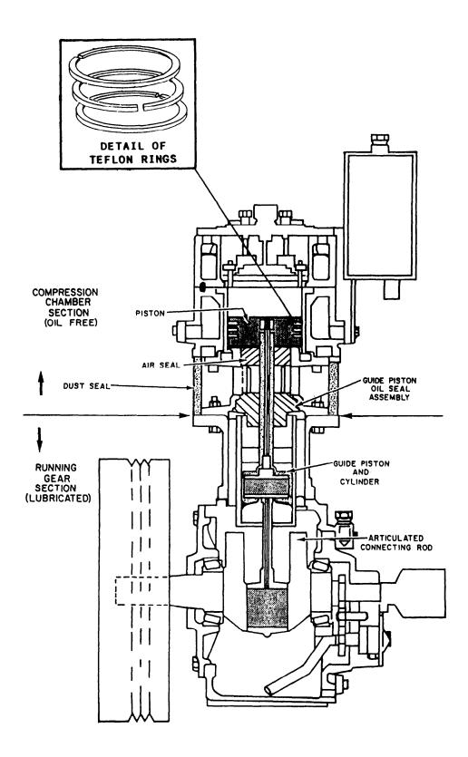
Figure 13-16.—Cut-away view of an oil free low-pressure air compressor.
