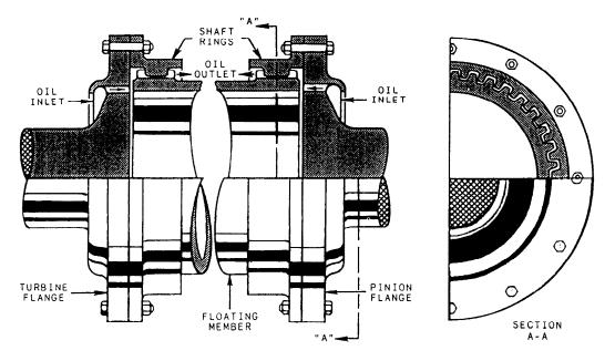
Figure 3-6.—Gear-type flexible coupling.
