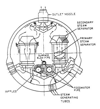
Figure 16-4.—Arrangement of steam drum internals in a single-furnace boiler.
