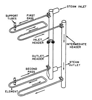
Figure 15-6.—Horizontal W-shaped tubes and steam flow through the superheater.
