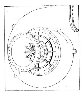
168.14 Figure 12-6.—Suction end of a centrifugal compressor showing prerotation vanes.
