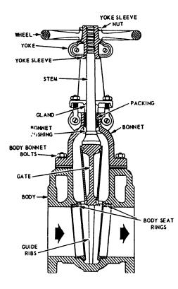
Figure 10-12.—Cutaway view of a gate stop valve (rising stem).
