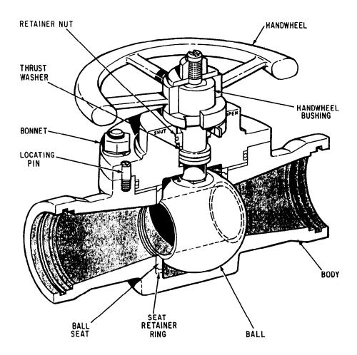
Figure 10-14.—Typical seawater ball valve.
