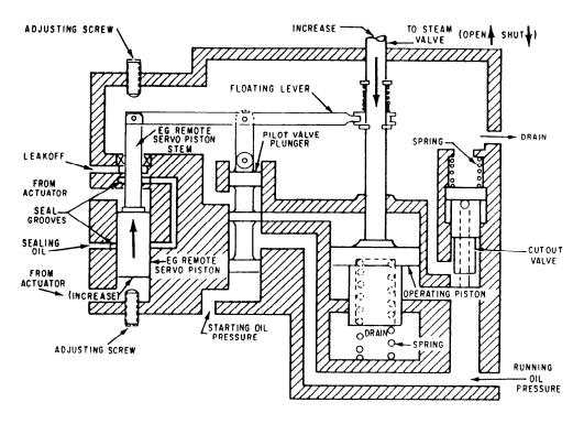
Figure 2-32.—Mechanical diagram of hydraulic valve operator.
