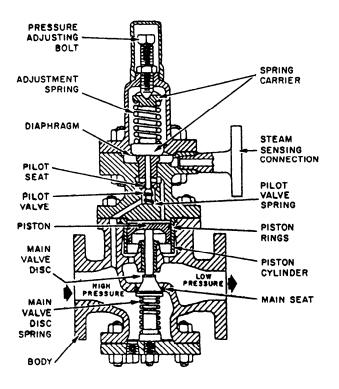
Figure 10-19.—Reducing valve (Atlas Valve Company).
