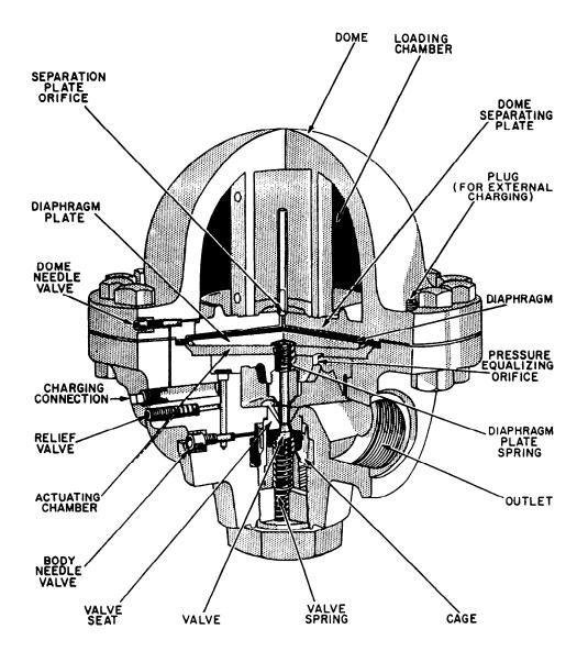
Figure 10-20.—Pneumatic-pressure-controlled reducing valve for low-temperature service.
