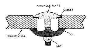
Figure 15-3.—Header handhole and handhole plate.
