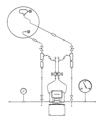
Figure 16-19.—Typical drum-level measurement installation for a second type of remote water-level indicator.
