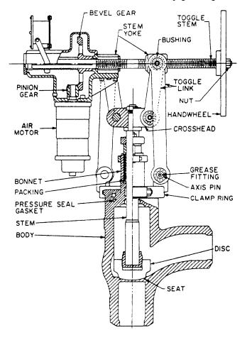
Figure 16-11.—Cross section of motor-operated gauge valve (main steam stop).
