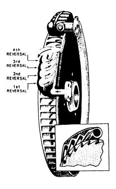
**33.45** Figure 2-13.—Cutaway view of steam path in a helical flow turbine.
