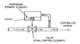
Figure 17-4.—Self-operated controller.
