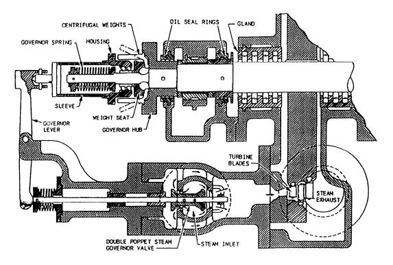
Figure 2-30.—Speed-limiting governor, main feed pump.
