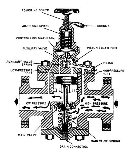
Figure 10-18.—Spring-loaded reducing valve.
