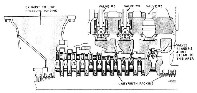
Figure 2-25.—High-pressure turbine showing valve arrangement.
