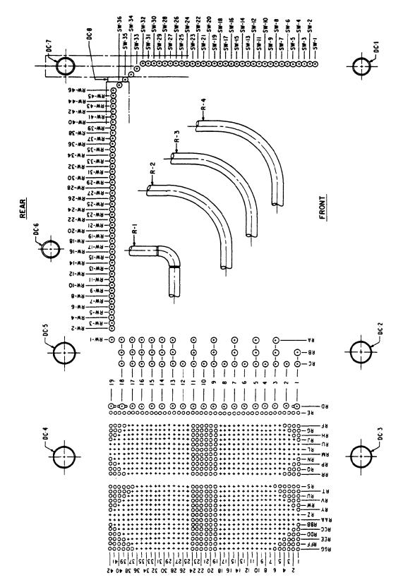
Figure 15-4.—Part of a boiler tube renewal sheet for a single-furnace boiler, showing tube identification.
