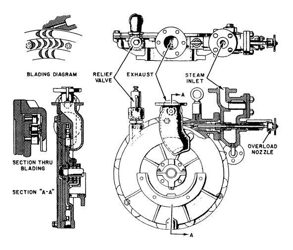
Figure 2-26.—Main lube oil pump turbine.
