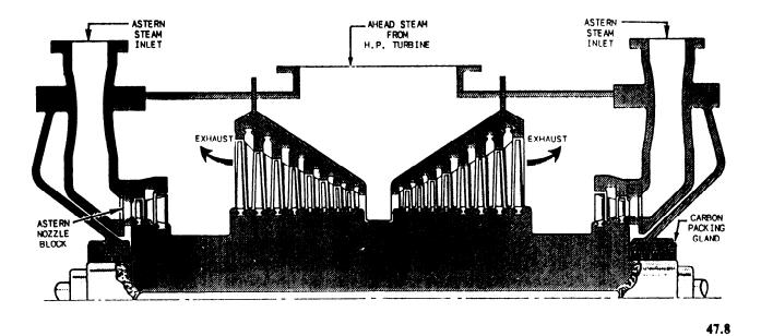
Figure 2-14.—Low-pressure double-axial flow reaction turbine.
