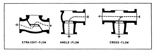
Figure 10-8.—Types of globe valve bodies.
