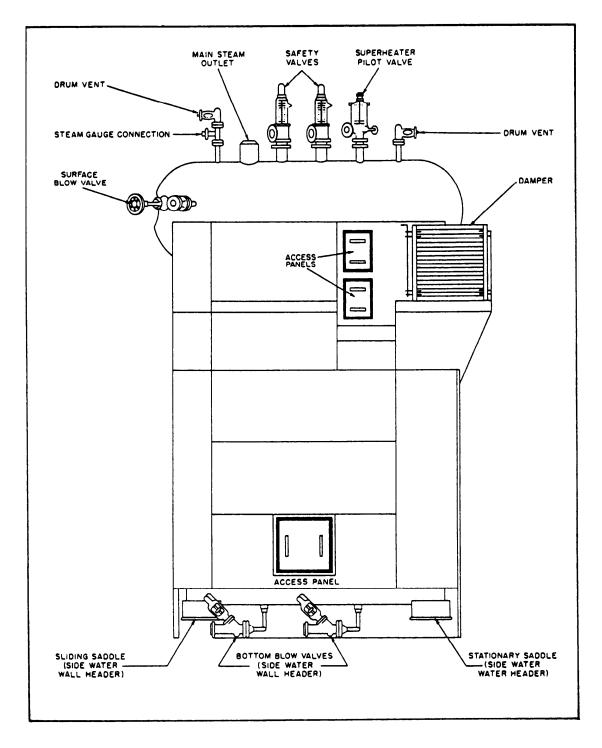
Figure 16-6.—External fittings and connections on a single-furnace boiler (side view).
