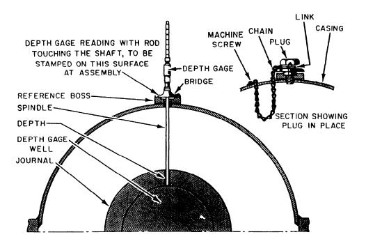
Figure 2-33.—Bearing wear micrometer depth gauge.
