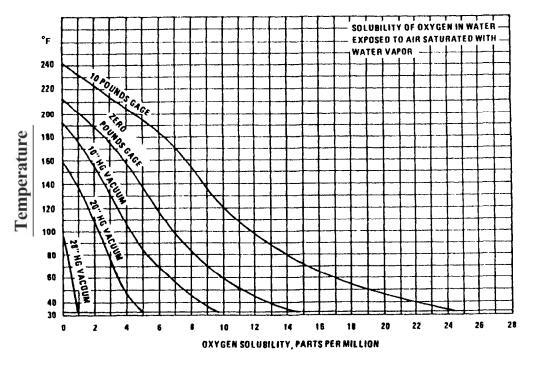
Figure 18-7.—Oxygen-dissolving capabilities of water.
