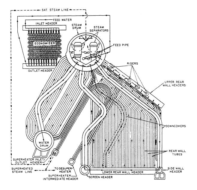
Figure 15-13.—Boiler water and steam flow.
