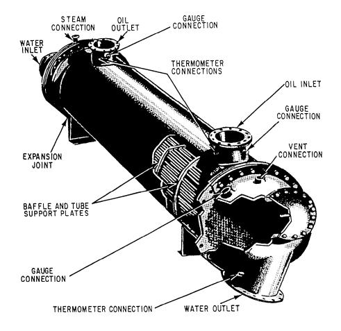
Figure 6-10.—Main lube oil cooler.
