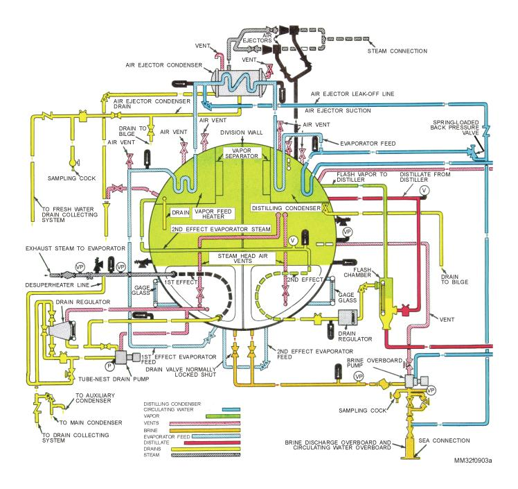
Figure 9-3.—Schematic diagram of a double-effect distilling plant.
