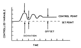
Figure 17-5.—Set point, deviation, control point, and offset in an automatic controller.
