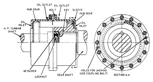
Figure 3-7.—Another gear-type flexible coupling.
