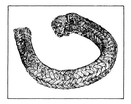
Figure 10-35.—Graphite filament yarn.
