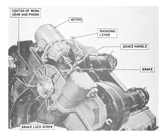
Figure 3-9.—Propulsion gear after end, high-pressure side, showing turning gear and propeller-locking mechanism.
