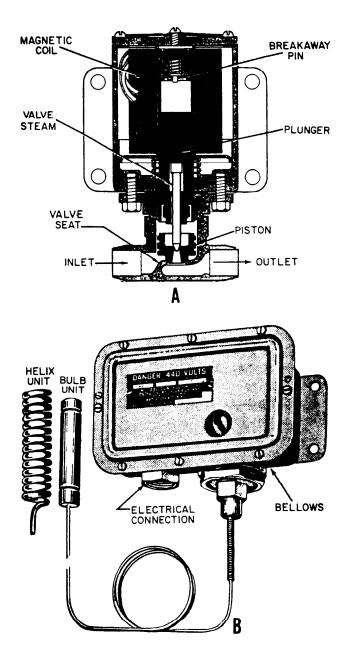
Figure 11-14.—Solenoid valve and thermostatic control switch.
