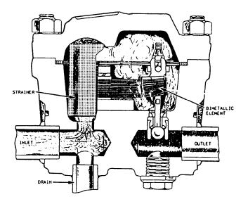
Figure 10-29.—Bimetallic steam trap.
