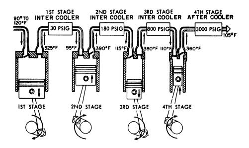
Figure 13-11.—Pressure and temperature resulting from multistaging and interstage cooling.
