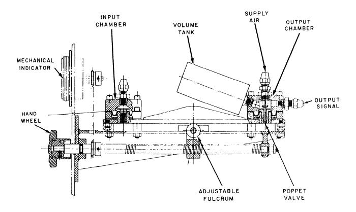
Figure 17-16.—F/A ratio signal generator (excess air adjuster).
