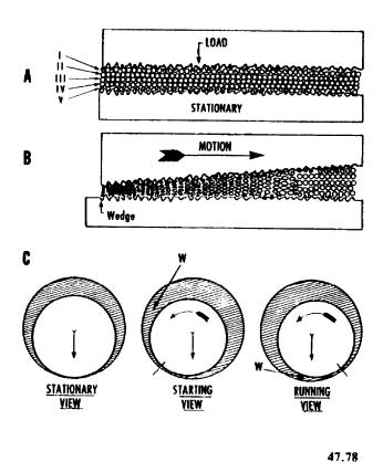
Figure 4-1.—Oil film lubrication.
