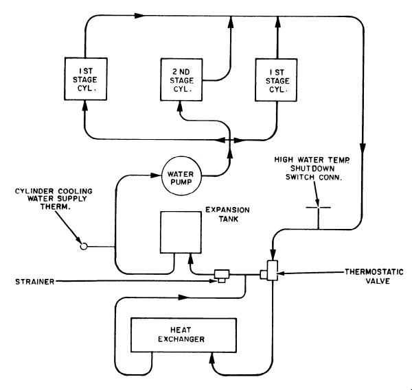
Figure 13-22.—Cylinder cooling water flow diagram.
