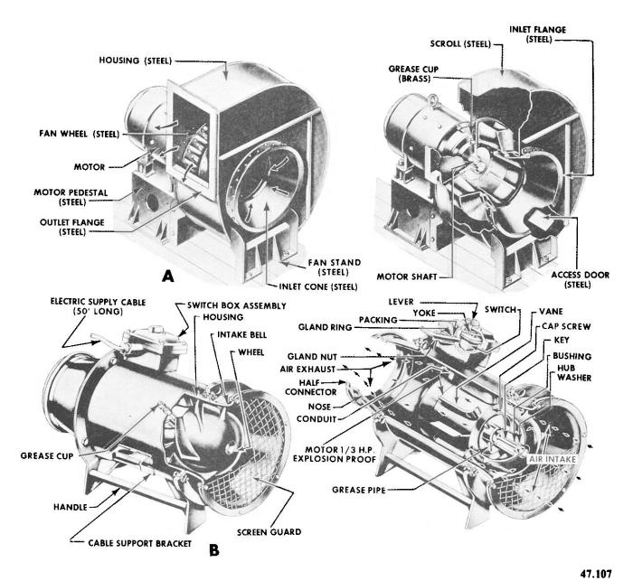
Figure 12-3.-Miscellaneous ventilating fans: A. Centrifugal fan. B. Portable axial fan.
