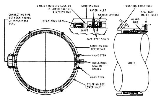
Figure 3-19.—Shaft seal and inflatable sealing ring.
