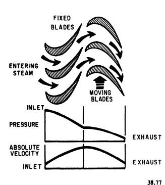
Figure 2-4.—Pressure-velocity relationship across reaction blading.
