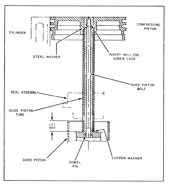
Figure 13-17.—Hollow-type piston assembly.
