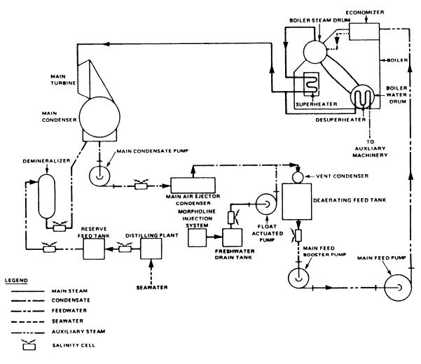
Figure 18-1.—Shipboard water cycle.
