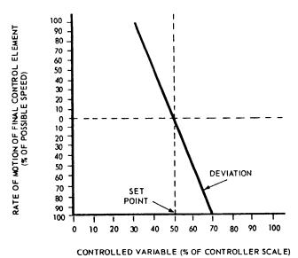
Figure 17-8.—Proportional-speed floating action.
