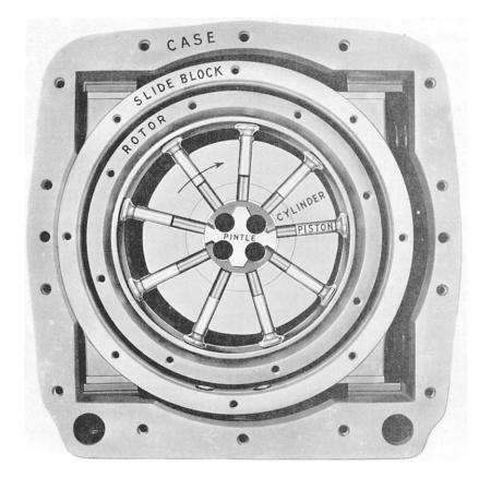
Figure 5-15.—Nine-piston radial piston pump.
