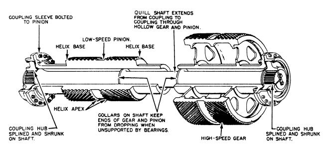
Figure 3-4.—Cutaway view of intermediate rotor assembly articulated gear.
