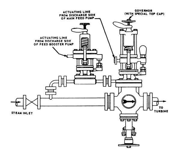
Figure 5-10.—Automatic shutdown device for main feed pump.
