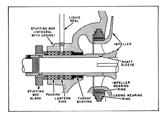
Figure 5-5.—Stuffing box on a centrifugal pump.
