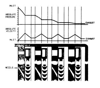
Figure 2-8.—Pressure-velocity relationships in a pressurecompounded impulse turbine.
