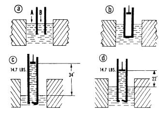
Figure 5-1.—Diagrams illustrating the principle of suction force.
