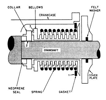
Figure 11-7.—Station bellows seal.
