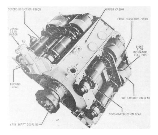
Figure 3-2.—Typical destroyer-type propulsion gear.
