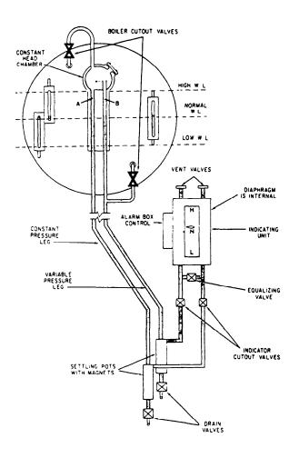
Figure 16-18.—General arrangement of a remote water-level indicator.
