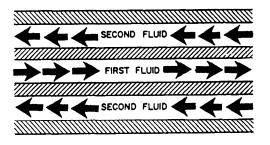
Figure 6-2.—Counterflow in a heat exchanger.
