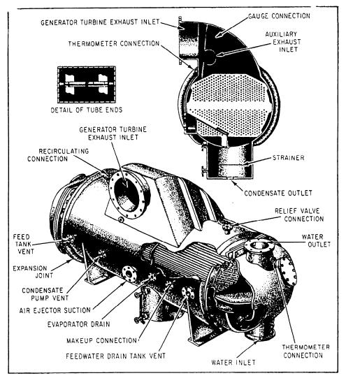
Figure 6-7.—Auxiliary condenser (turbogenerator).
