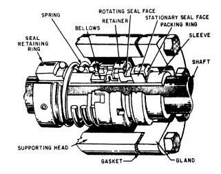
Figure 5-6.—Type-1 mechanical seal.
