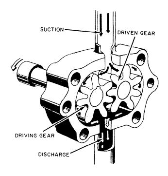
Figure 5-16.—Simple gear rotary pump.
