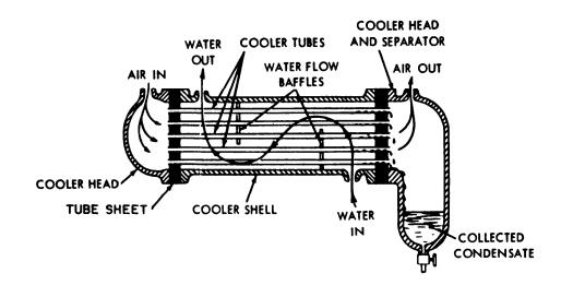
Figure 13-10.—Basic cooler and separator.
