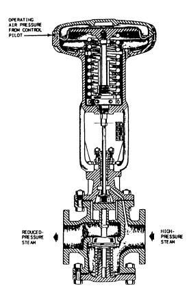
Figure 10-23.—Diaphragm control valve (upward seating).
