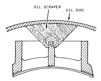
Figure 3-17.—Disc-oiled line shaft bearing scraper arrangement.
