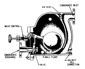
Figure 10-26.—A ball-float steam trap.
