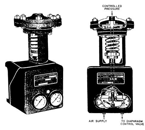
Figure 10-21.—Air-operated control pilot.
