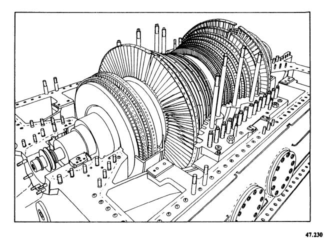
Figure 2-23.-L. P. turbine cylinder base with rotor installed, viewed from thrust end.
