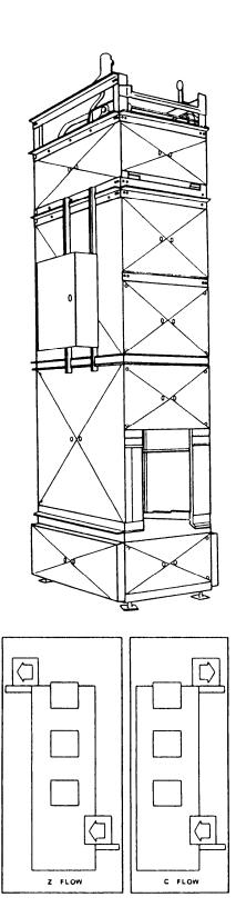
Figure 14-7.—Vertical conveyor, pallet, tray type.
