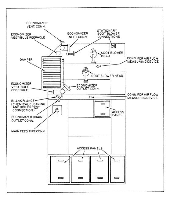
Figure 16-7.—External fittings and connections on a single-furnace boiler (economizer side view).
