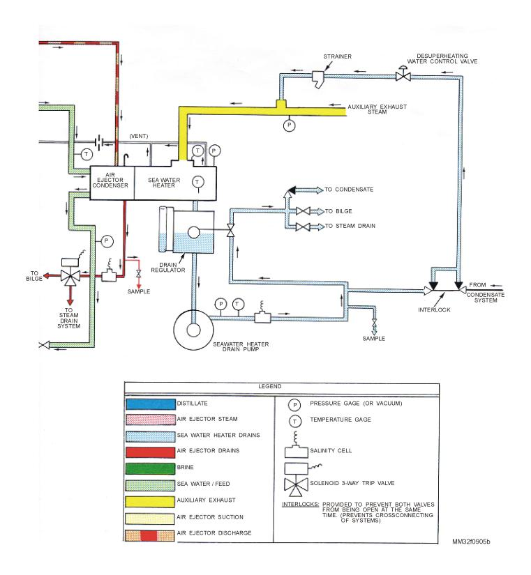
Figure 9-5.—Two-stage, flash-type distilling plant 12,000 gpd capacity-(cont)
