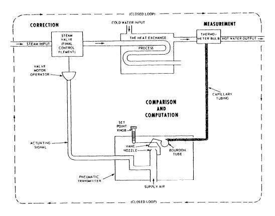
Figure 17-3.—Simple automatic control system (pneumatic) for control of heat exchange process.
