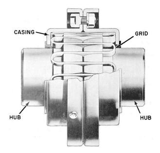
Figure 5-7.—Grid-type flexible coupling.
