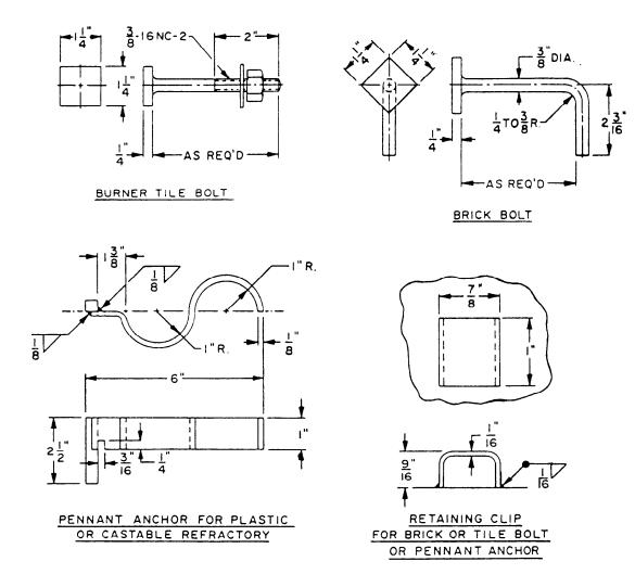
Figure 15-10.—Refractory anchor devices.
