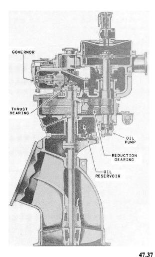
Figure 3-10.—Vertical propeller type of main condenser circulating pump.
