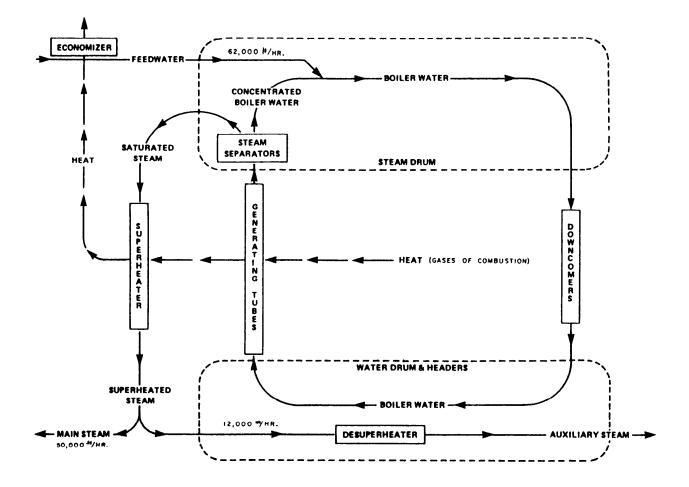
Figure 18-2.—Propulsion boiler water flow.
