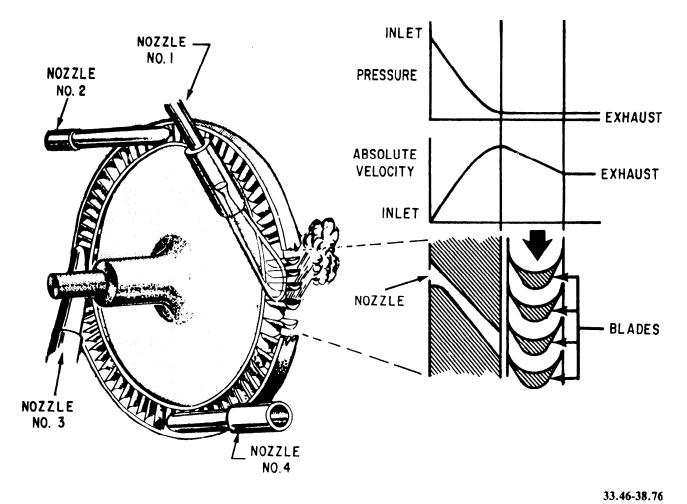
Figure 2-3.—Pressure-velocity relationship across the nozzles and moving blades of an impulse type turbine.
