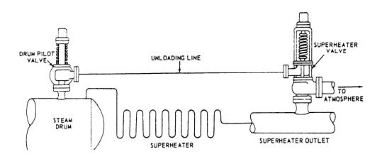
Figure 16-23.—Two-valve superheater outlet safety valve assembly.
