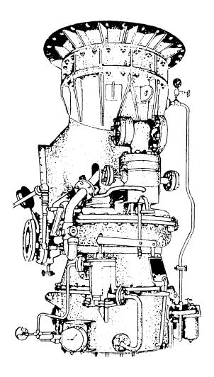
Figure 5-25.—View of a two-stage vertical propeller-type blower from the steam chest side.
