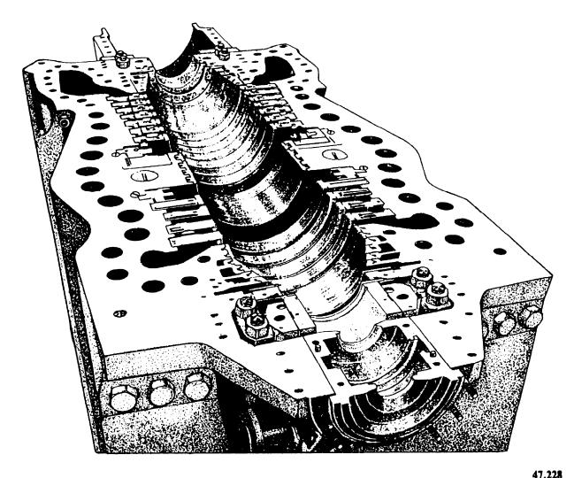
Figure 2-18.—HP-IP turbine cylinder base with lower sections of seals and diaphragms installed, viewed from thrust end.
