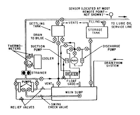
Figure 4-2.—Typical lube oil system.
