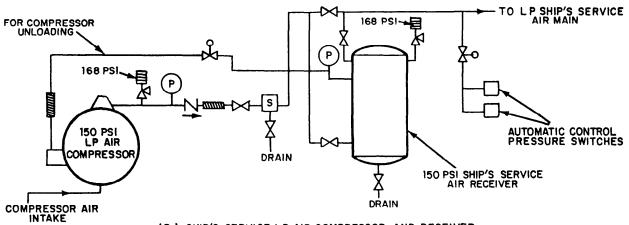
(B) SHIP'S SERVICE LP AIR COMPRESSOR AND RECEIVER
