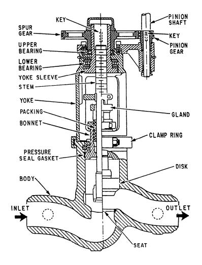
Figure 10-10.—Gear-operated globe stop valve.
