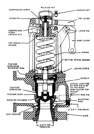
Figure 16-21.—Steam drum safety valve (huddling-chamber type).
