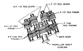
Figure 3-1.—Articulated locked train, double-reduction gear.
