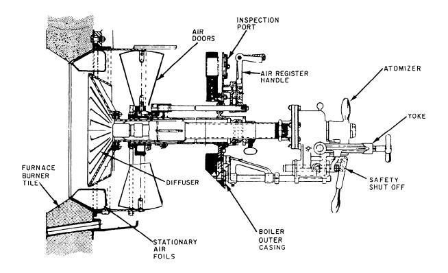
Figure 16-29.—Fuel-oil burner assembly.
