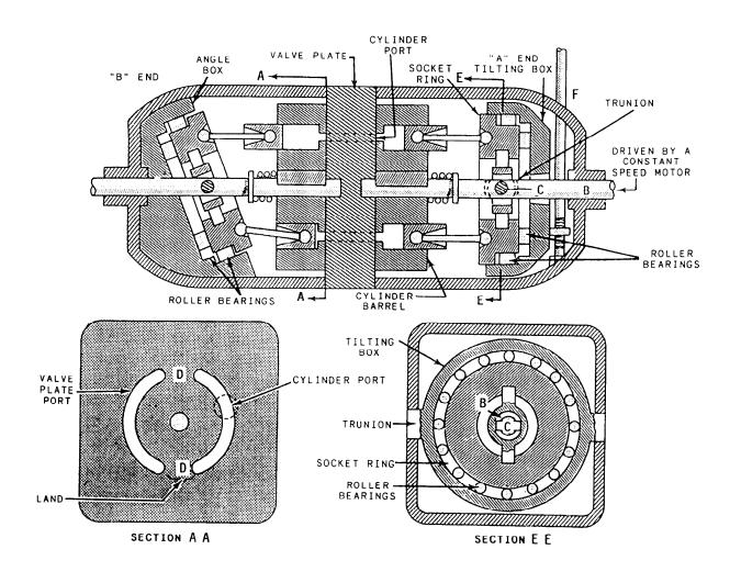
Figure 5-14.—Axial piston hydraulic speed gear.
