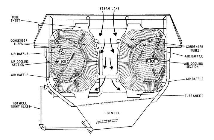
Figure 6-6.—Cross-sectional view of the internals of a main condenser.
