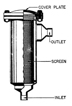
Figure 11-17.—Strainer of liquid refrigerant.
