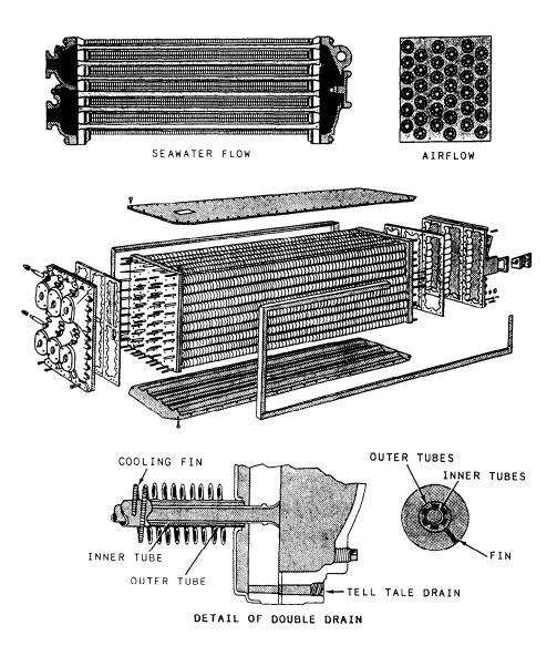
Figure 6-12.—Air cooler for a motor generator.
