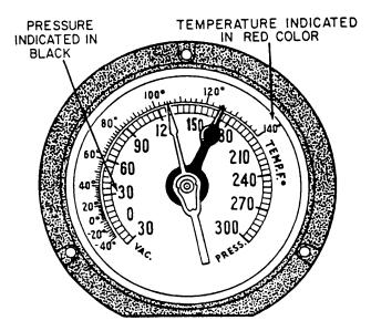
Figure 11-18.—Compound R-12 pressure gauge.
