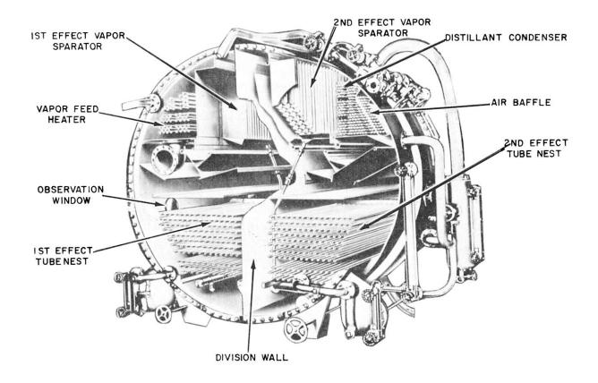
Figure 9-2.—Internal construction of a double-effect distilling plant.
