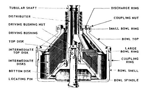
Figure 4-6.—Part of a disk-type purifier bowl.
