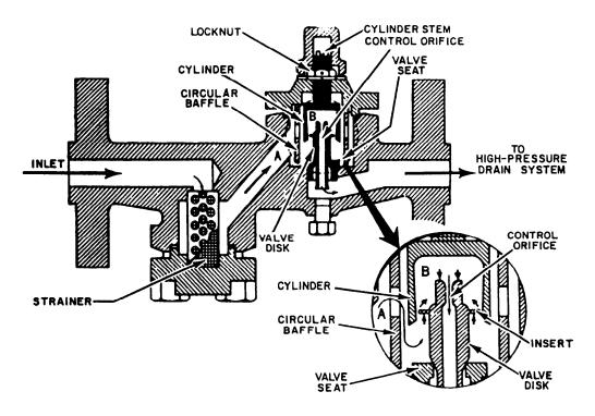
Figure 10-28.—Impulse steam trap.
