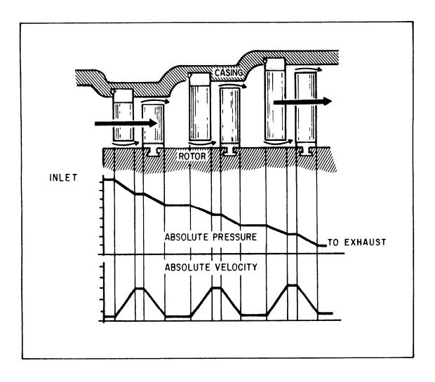
Figure 2-10.—Diagrammatic arrangement of reaction blading showing velocity and pressure relationships.
