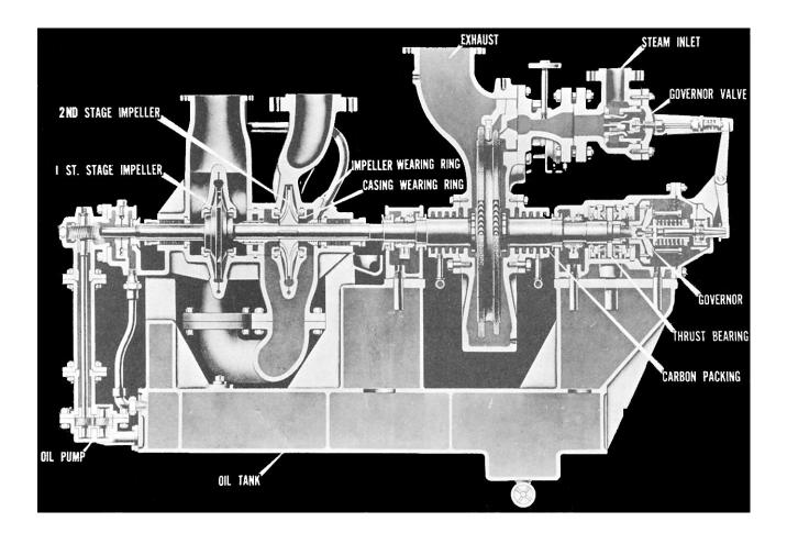
Figure 5-4.—Two-stage main feed pump.
