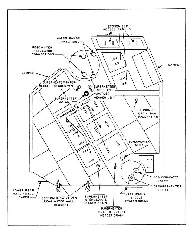
Figure 16-8.—External fittings and connections on a single-furnace boiler (rear view).
