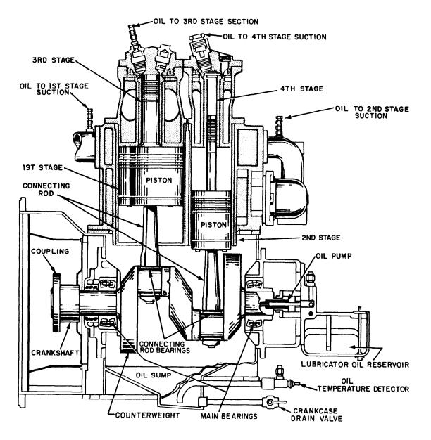
Figure 13-7.—High-pressure air compressor.
