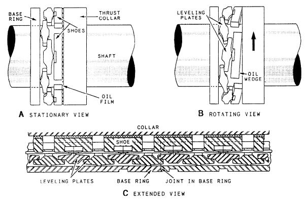
Figure 3-14.—Diagrammatic arrangement of a typical thrust bearing.
