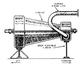
47.12 Figure 2-15.—Turbine foundation, showing flexible I-beam.
