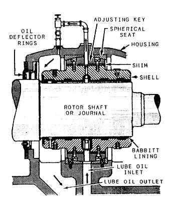
Figure 4-4.—Adjustable spherical-seated bearing lubricated by force feed.
