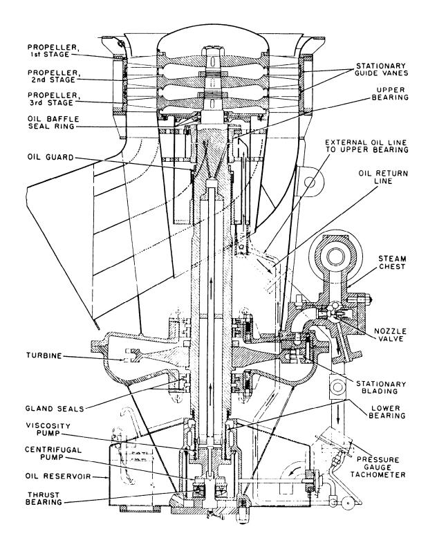
Figure 5-27.—Sectional view of a three-stage vertical propeller-type blower.
