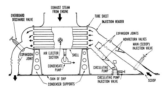
Figure 6-4.—Schematic arrangement of a main condensing system.
