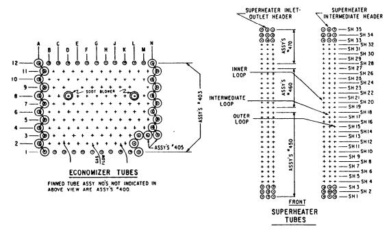
Figure 15-5.—Part of a boiler tube renewal sheet for a single-furnace boiler, showing tube identification.
