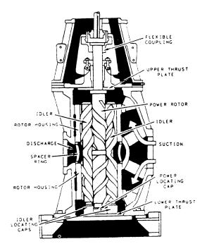
Figure 5-20A.—Triple-screw high-pitch pump.
