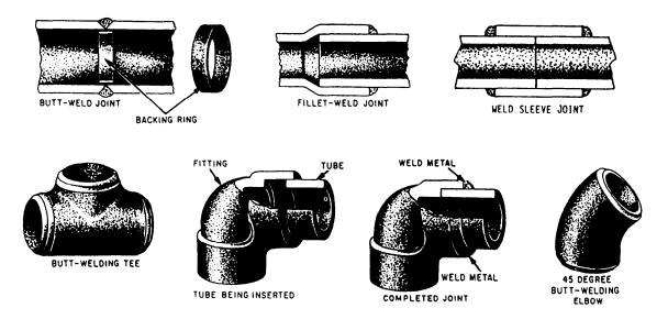
Figure 10-3.—Various types of welded joints.
