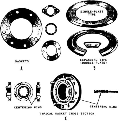
Figure 10-36.—Fixed joint gaskets. A. Sheet asbestos gaskets. B. Serrated-face metal gasket. C. Spiral-wound metallic asbestos gasket.
