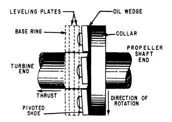
Figure 3-12.—Diagrammatic arrangement of a pivoted-shoe thrust bearing showing oil film.
