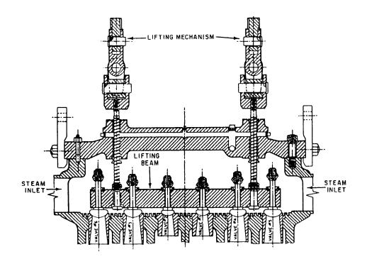
Figure 2-24.—Arrangement of nozzle control valves.
