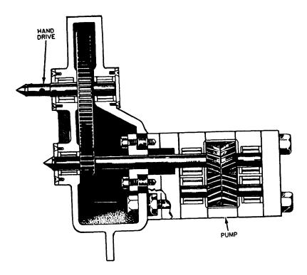
Figure 5-17.—Herringbone gear pump.
