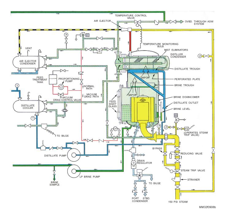
Figure 9-8.—Single-stage, vertical basket distilling plant 8,000 gpd capacity-(cont)
