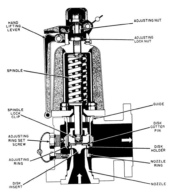
Figure 16-22.—Steam drum safety valve (nozzle-reaction type).
