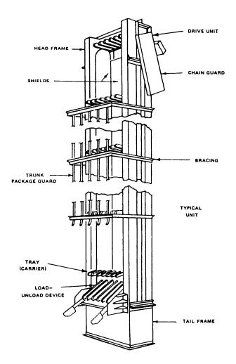
Figure 14-6.—Vertical conveyor, package, tray type.
