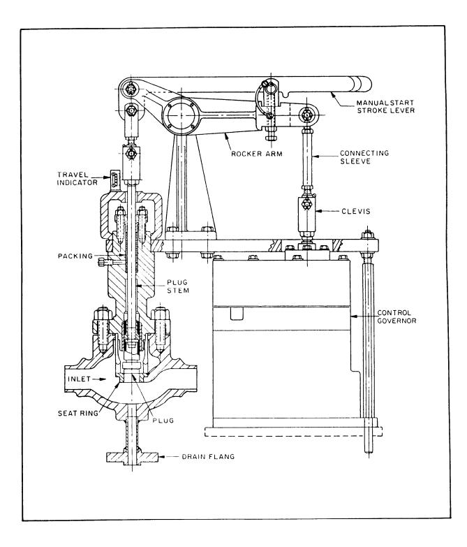
Figure 5-24.—Steam inlet valve.
