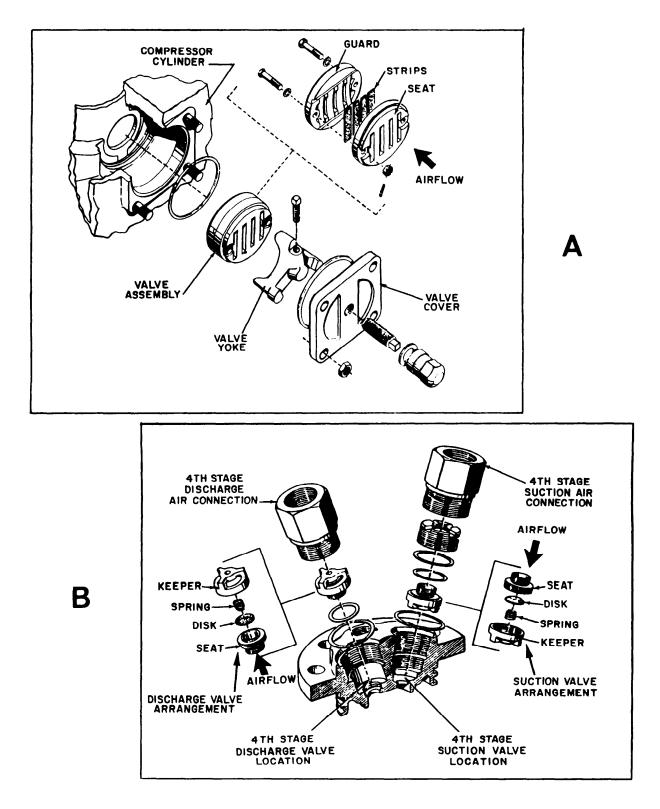
Figure 13-5.—High-pressure air compressor valves: (A) Valve arrangement for lower pressure stages (suction shown); (B) Valve arrangement for higher pressure stages (both suction and discharge shown).
