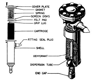
Figure 11-13.—Refrigeration dehydrator.
