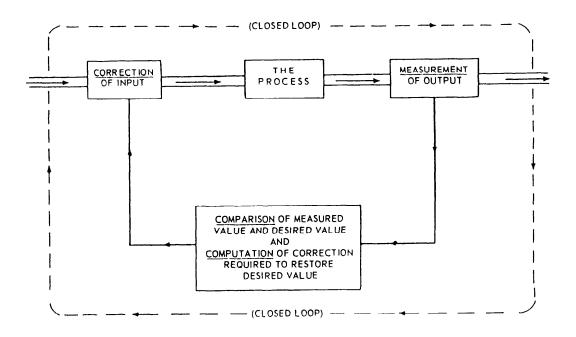
Figure 17-2.—Closed loop of control.
