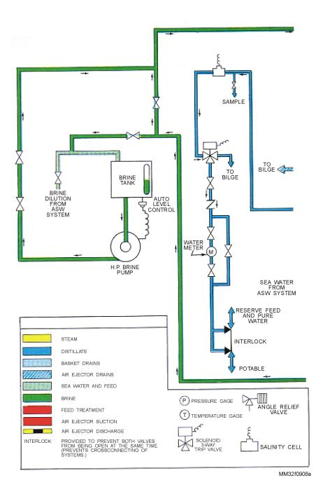
Figure 9-8.—Single-stage, vertical basket distilling plant 8,000 gpd capacity.
