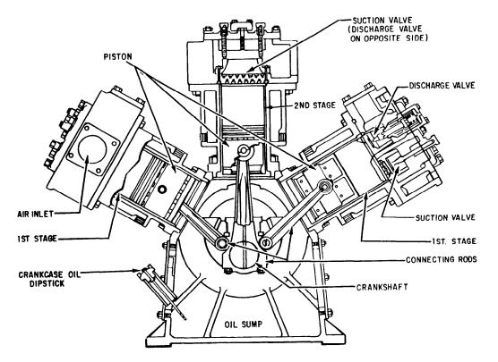
Figure 13-2.-Low-pressure reciprocating air compressor, vertical W configuration.
