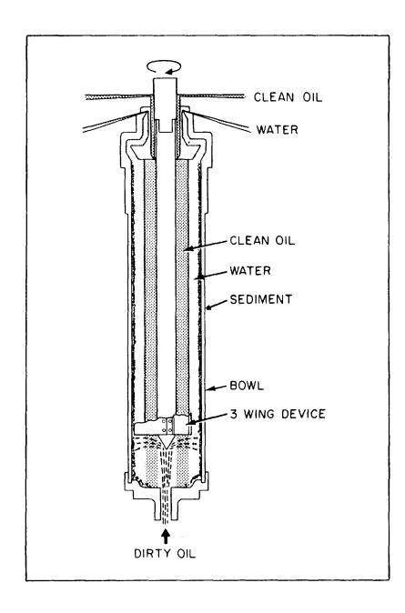
Figure 4-9.—Principles of a centrifugal purifier.
