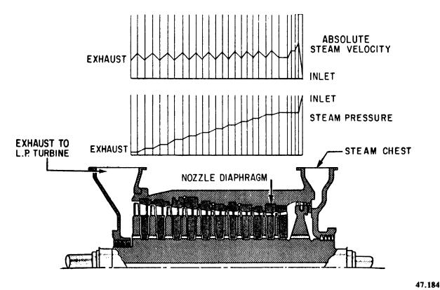
Figure 2-9.—Pressure-velocity-compounded impulse turbine showing velocity and pressure relationships.
