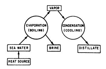
Figure 9-1.—Simplified diagram of shipboard distillation process.
