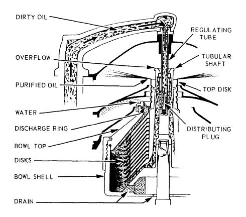
Figure 4-7.—Path of oil through disk-type purifier.
