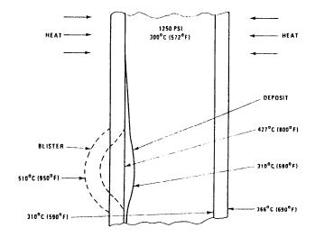
Figure 18-6.—Effect of boiler deposit.
