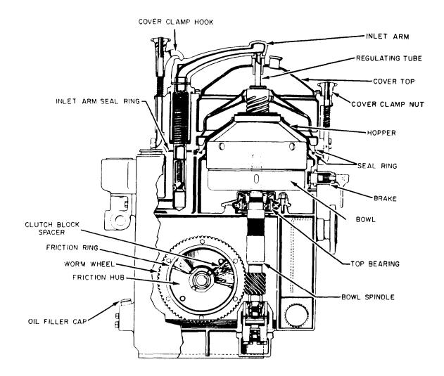
Figure 4-5.—Disk-type centrifugal purifier.
