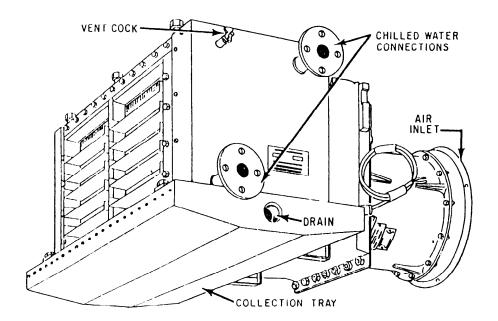
Figure 12-9.—Fan-coil assembly.
