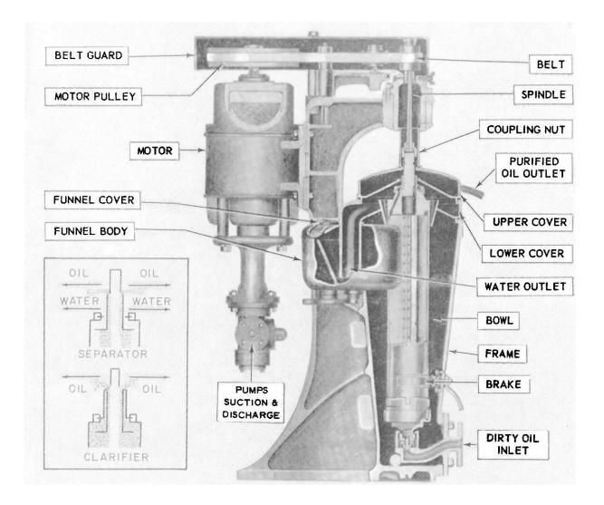
Figure 4-8.—Tubular-type centrifugal purifier.
