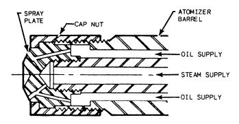
Figure 16-27.—Y-jet steam atomizer.
