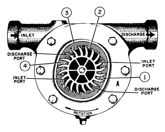
Figure 13-13.—Rotary-centrifugal compressor.
