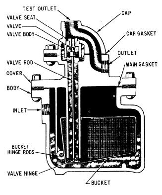
Figure 10-27.—Bucket-type steam trap.
