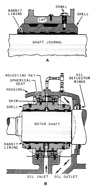
Figure 3-11.—Turbine rotor bearings. A. Cylindrical-seated bearing. B. Adjustable spherical-seated bearing.
