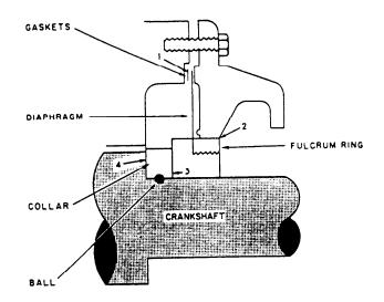
Figure 11-9.—Diaphragm-type seal.
