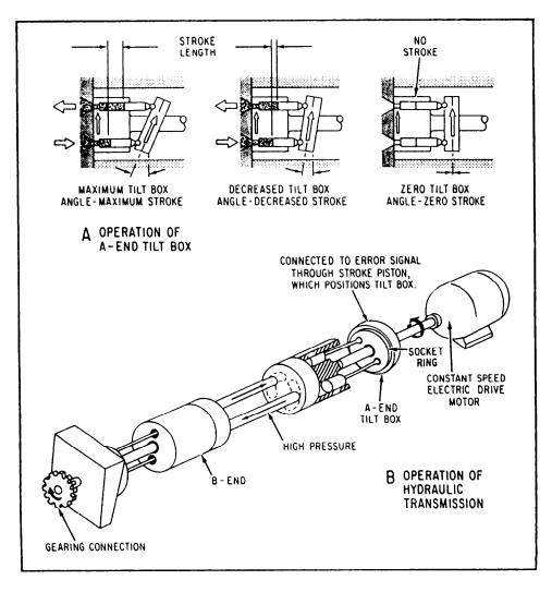
Figure 14-1.—Electrohydraulic speed gear.
