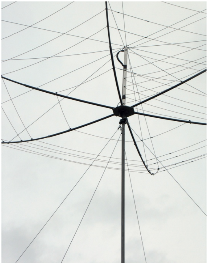
Two sets of guy wires attach to bushings allowing the mast to rotate.
