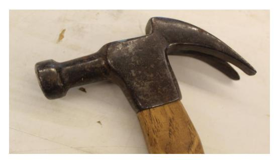
Hammer with offset fulcrum. From "The Hammer, the King of Tools" by Baird and Comerford. Conrad Berthold
