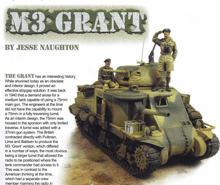
omitted the small machine gun turret on top, which lowered the tank by almost a foot. There were some internal changes as well to ammo stowage and other details and these were further modified throughout the vehicle's life cycle.
