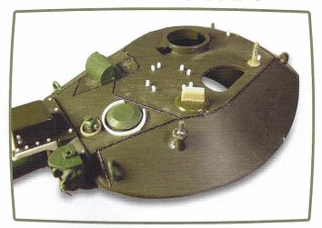
I added detail to the gun shield such as the searchlight mount and the cover for the gun sight.
